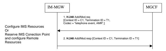
Figure 49: Activation of processing of DTMF digits received in RTP for sending the digits inband to CS CN (message sequence chart)
