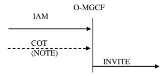
NOTE: Waiting for the COT is recommended, if the Continuity Check indicator in the Nature of Connection Indicators parameter in the incoming IAM is set to indicate either "continuity check required on this circuit" or "continuity check performed on previous circuit"
