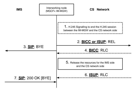
NOTE: Signal 6 is omitted when IM CN subsystem interworks with BICC based CS network and Signal 4 is omitted when IM CN subsystem interworks with ISUP based CS network.
