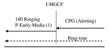
NOTE 1: The P-Early-Media header field is included if the received INVITE contains a P-Early-Media header field with the "supported" parameter as described in IETF RFC 5009 [89].
