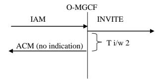
Figure 17: Sending of ACM (Ti/w<sub>2</sub> elapses)
