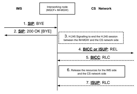
NOTE: Signal 7 is omitted when IM CN subsystem interworks with BICC based CS network and Signal 5 is omitted when IM CN subsystem interworks with ISUP based CS network.
