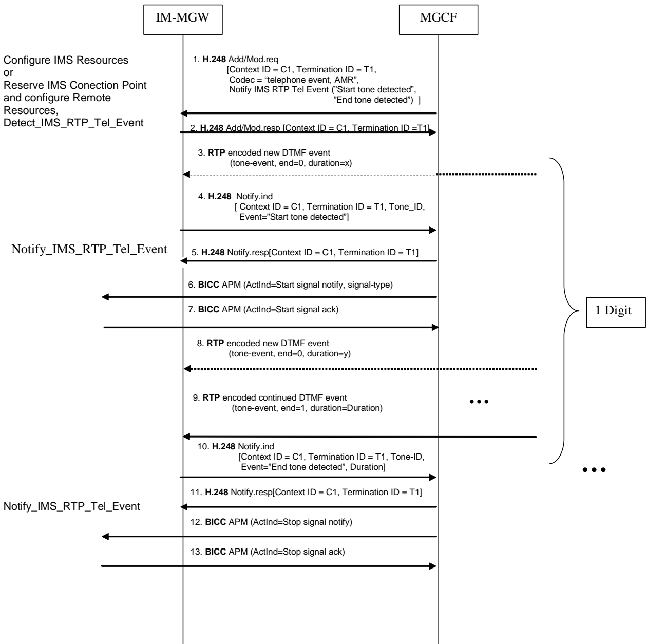
Figure 48a: Activation of notification of DTMF digits received in RTP and examples of sending the digits out-of-band to CS CN, IM-MGW starts sending the digit further when the start of the digit is recognized (message sequence chart)
