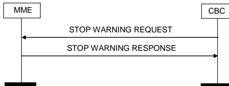
Figure 4.3.3A.2-1: Stop Warning Procedure, Successful Operation.
