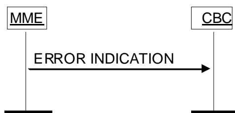
Figure 4.3.3B.2-2: Error Indication procedure, MME originated. Successful operation.
