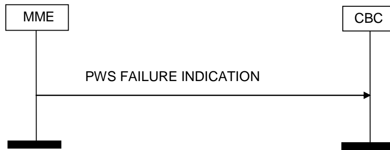
Figure 4.3.3F.2-1: PWS Failure Indication, Successful Operation.
