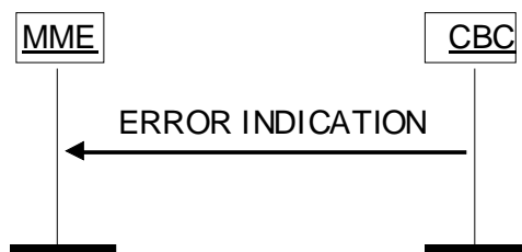
Figure 4.3.3B.2-1: Error Indication procedure, CBC originated. Successful operation.
