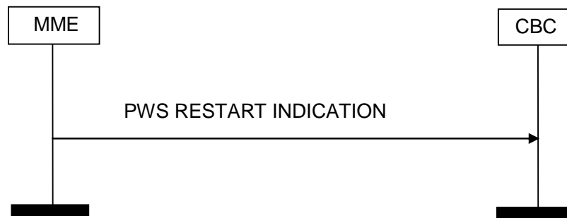
Figure 4.3.3E.2-1: PWS Restart Indication, Successful Operation.
