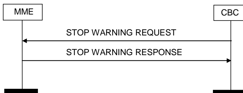
Figure 4.3.3A.3-1: Stop Warning procedure, Unsuccessful operation.
