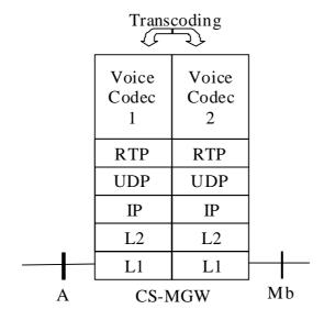
Figure 6.4.1.1: IP-based A to Mb protocol stack (transcoding)
