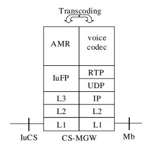
Figure 6.2.1.1: luCS to Mb protocol stack (transcoding)
