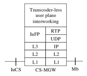
Figure 6.2.2.1: IuCS to Mb protocol stack (no transcoding)
