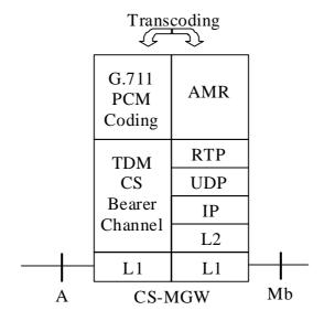
Figure 6.3.1.1: TDM-based A to Mb protocol stack (transcoding)
