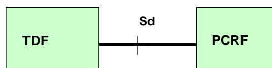
Figure 4b.2.1: Sd reference model
