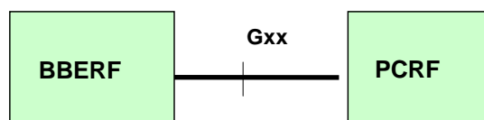
Figure 4a.2.1: Gxx reference model
