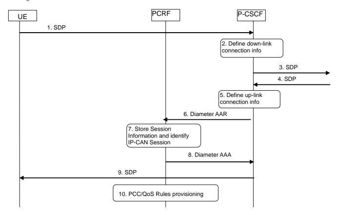
Figure B.2.1.1: PCC Procedures for IMS Session Establishment at originating P-CSCF and PCRF
