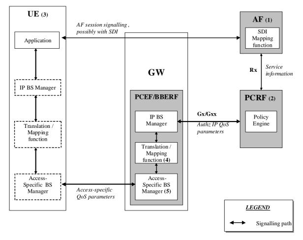
Figure 6.1.1: Framework for QoS mapping
