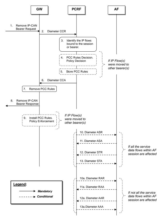
Figure D.3.1.2.2: UE-Initiated IP-CAN Bearer Termination
