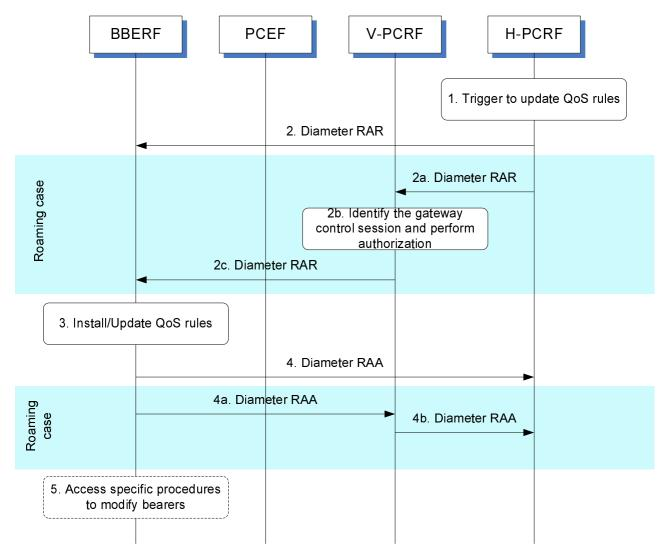
Figure 4.4.3.1: Gateway Control and QoS Rules Provision
