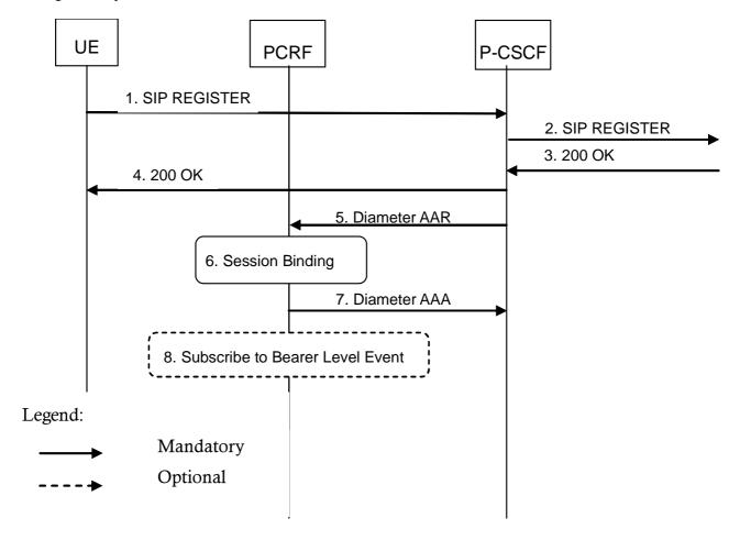
Figure B.1.1: Subscription to Notification of IMS Signaling Path Status at initial IMS Registration
