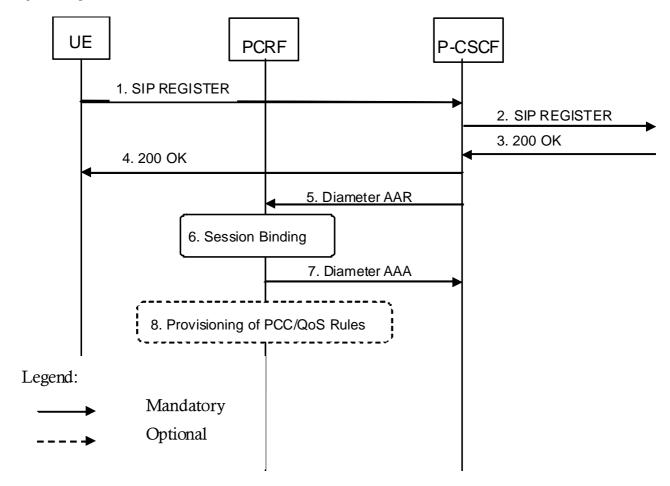
Figure B.1.3: Provisioning of SIP Signalling Flow Information at initial IMS Registration
