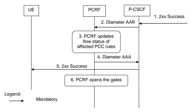
Figure B.3.2.1: Enabling of IP Flows
