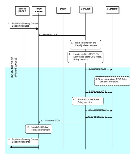
Figure 4.5.2.1.1: Gateway Control Session Establishment during BBERF relocation.
