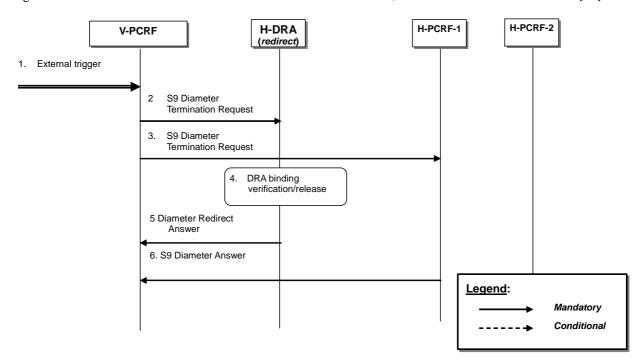
Figure 7.4.2.3.2.1: Termination of Diameter sessions through DRA (redirect) - Roaming case
