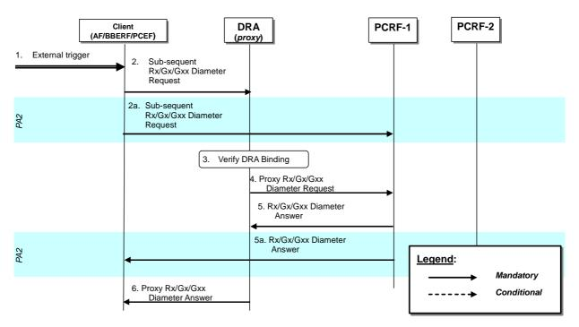
Figure 7.4.1.2.1.1.1: Modification of Diameter sessions through DRA (proxy)- AF/BBERF/PCEF interaction
