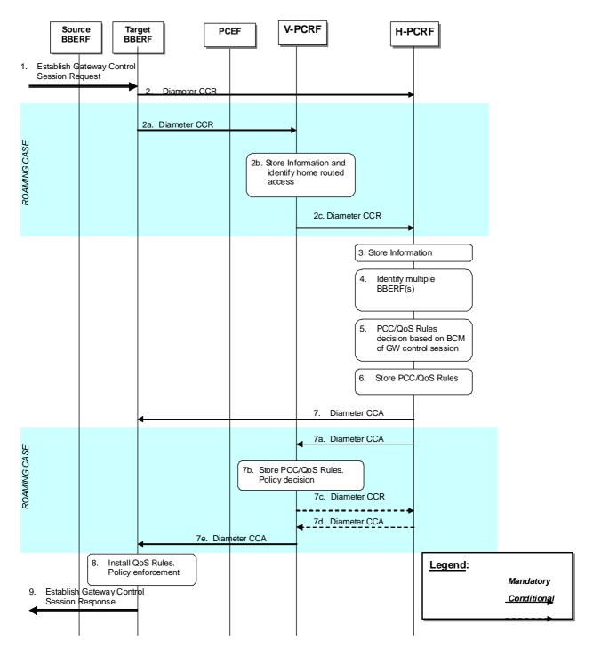
Figure 4.5.1.1.1: Gateway Control Session Establishment during BBERF relocation.
