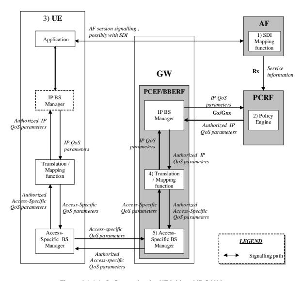
Figure 6.1.1.1: QoS mapping for UE initiated IP CAN bearers
