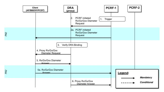
Figure 7.4.1.2.1.2.1: Modification of Diameter sessions through DRA (proxy)- PCRF interaction
