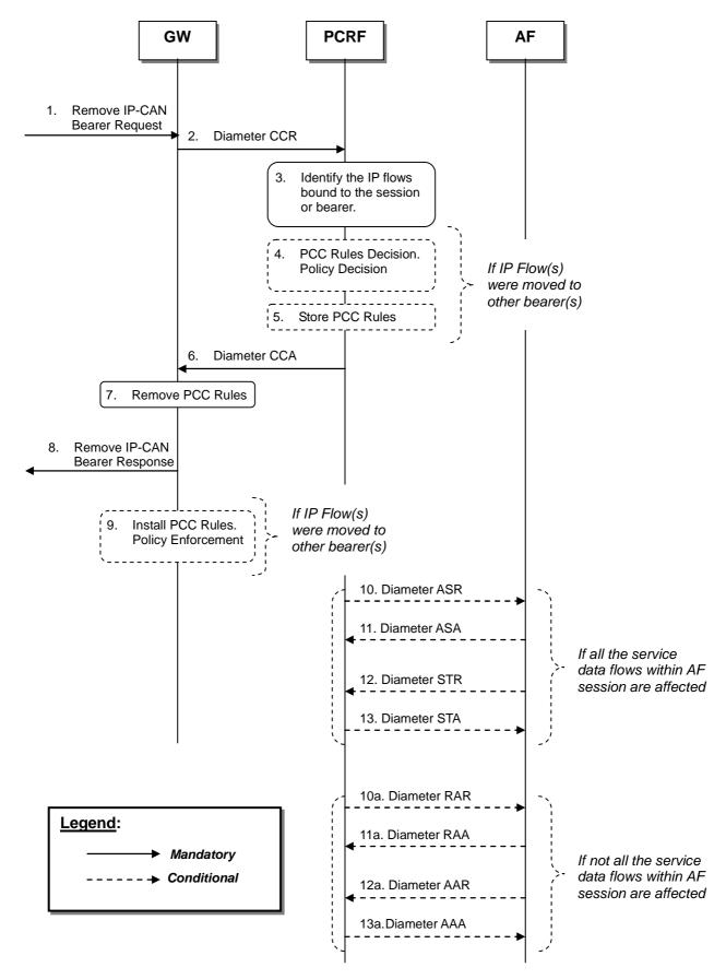
Figure D.3.1.2.2: UE-Initiated IP-CAN Bearer Termination
