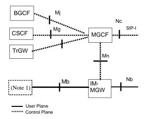
NOTE 1: The IM-MGW may be connected via the Mb to various network entities, such as a UE (via a GTP Tunnel to a GGSN), an MRFP, or an application server.
