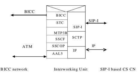
Figure 6.2.2: Control plane interworking between SIP-I based CS CN and a BICC based network with ATM signalling transport
