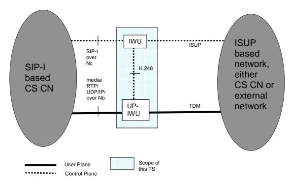
NOTE: The IWU is a logical function that may reside with other 3GPP logical functions in the same physical nodes, e.g. in an (G)MSC Server. The figure shows only the logical separation.
