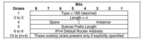
Figure 8. 97-1: IPv4 Configuration Parameters (IP4CP)
