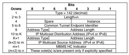
Figure 8.73-1: MBMS IP Multicast Distribution
