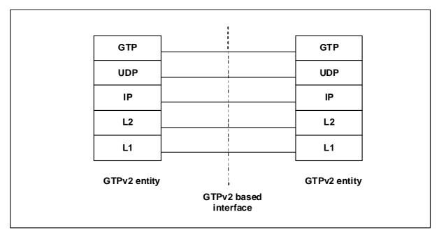
Figure 4.2.0-1: GTPv2 stack
