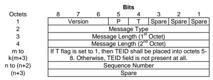
Figure 5.1-1: General format of GTPv2 Header for Control Plane
