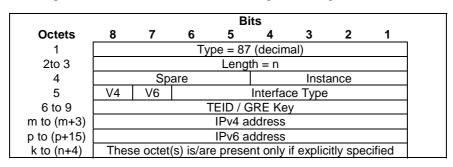
Figure 8.22-1: Fully Qualified Tunnel Endpoint Identifier (F-TEID)
