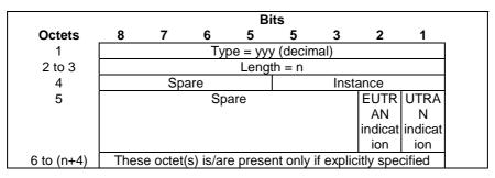
Figure 8.116-1: WLAN Offloadability Indication
