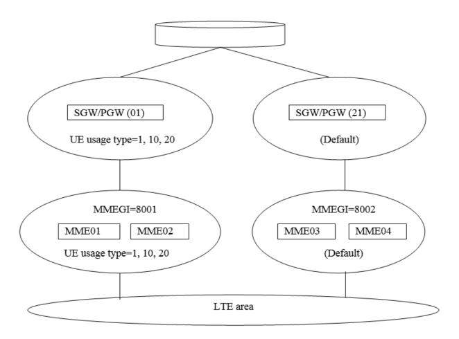
Figure A.4.x1-1: Simple example of DCN depolyment
