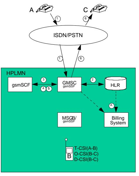
Figure 5.21: Incoming call handled by CAMEL with redirection decided and forwarding leg handled by CAMEL with Dialled CSI Trigger
