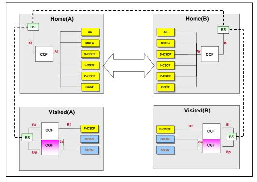
Figure 4.5 presents the off-line IMS charging architecture for roaming scenario.
