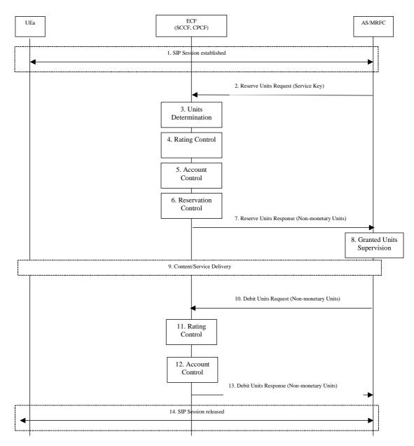
Figure 7.5: Event Charging with Reservation / Centralized Unit Determination and Centralized Rating
