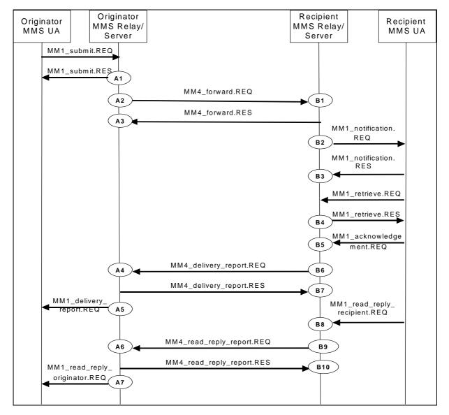
Figure 8.2: Record trigger overview for distributed case
