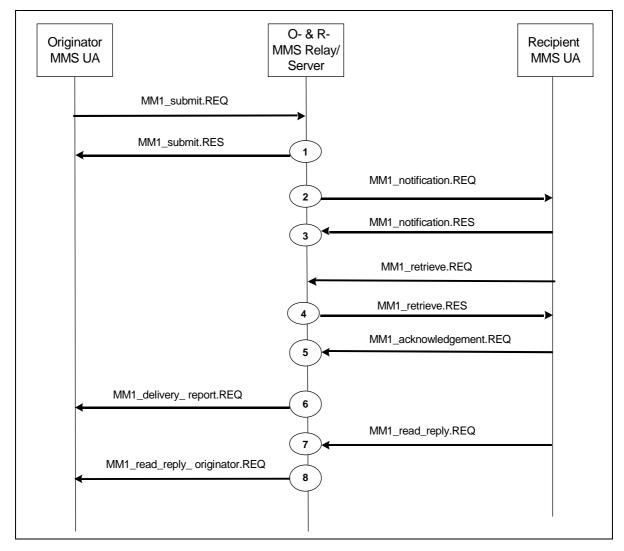
Figure 8.1: Record trigger overview for combined case
