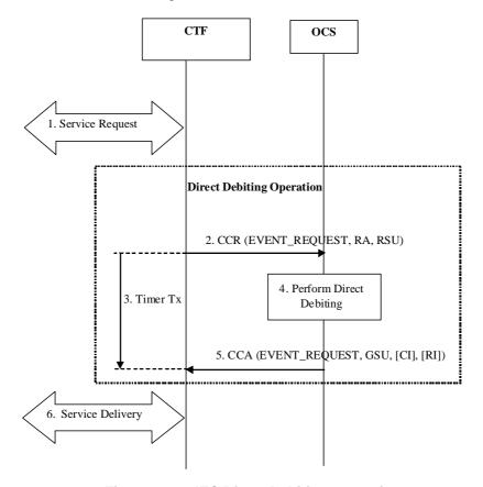
Figure 6.3.3: IEC Direct Debiting Operation
