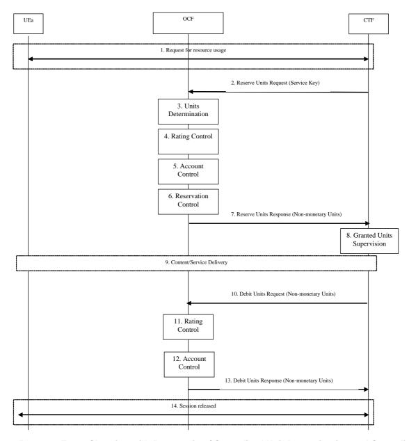
Figure 5.2.2.2: Event Charging with Reservation / Centralized Unit Determination and Centralized Rating
