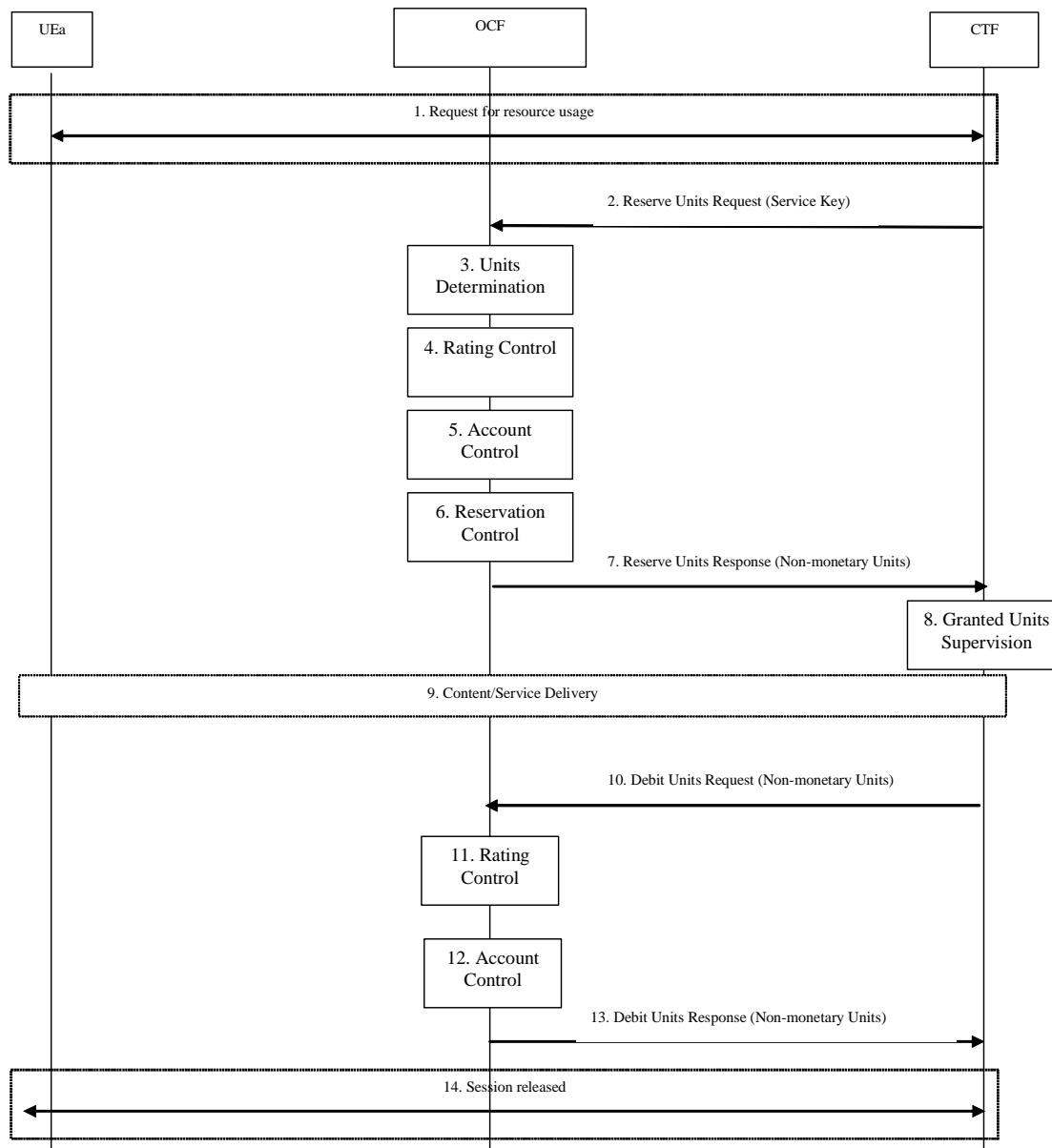
**Figure 5.2.2.2.2.1: ECUR - Centralized Unit Determination and Centralized Rating**
