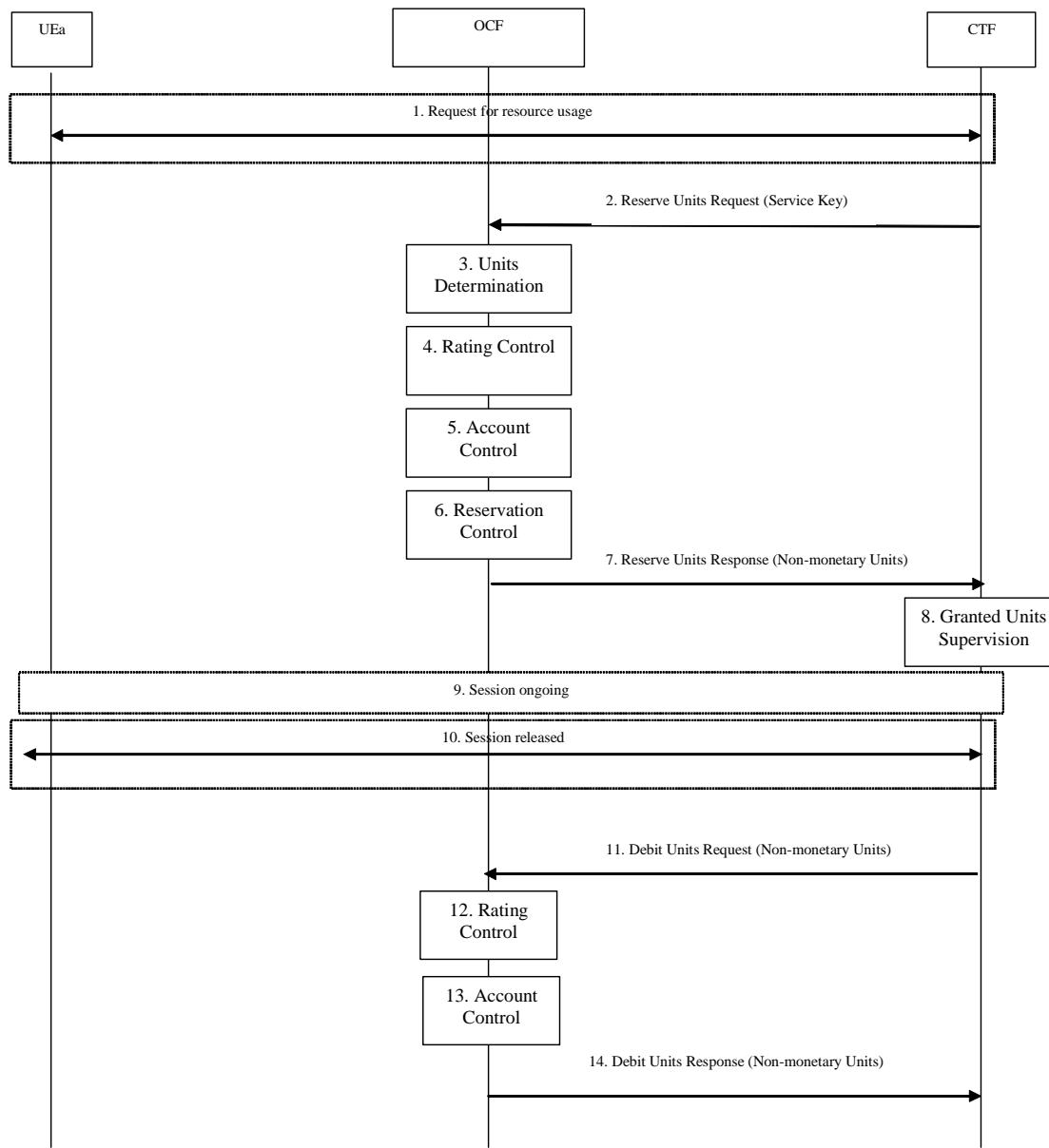
**Figure 5.2.2.3.2.1: SCUR - Centralized Unit Determination and Centralized Rating**
