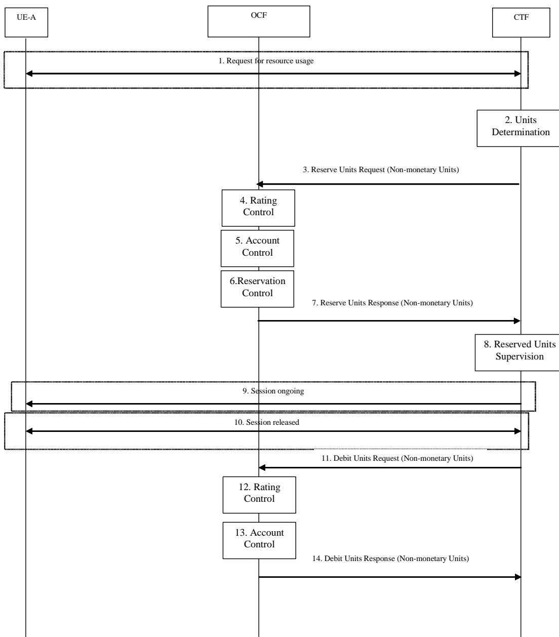
**Figure 5.2.2.3.1.1: SCUR - Decentralized Unit Determination and Centralized Rating**
