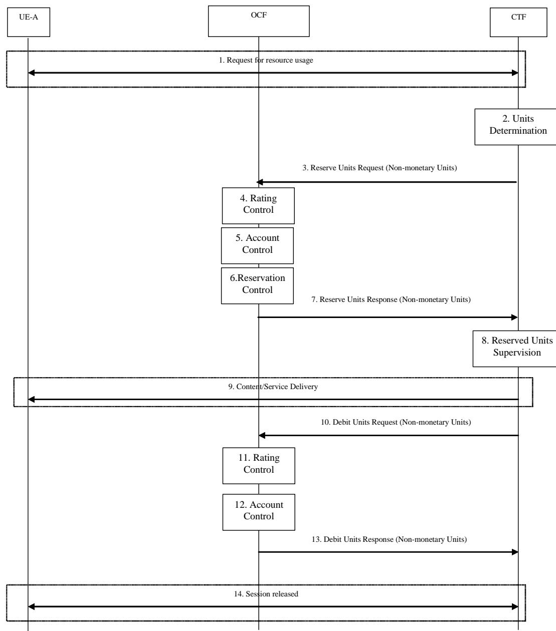
**Figure 5.2.2.2.1.1: ECUR - Decentralized Unit Determination and Centralized Rating**
