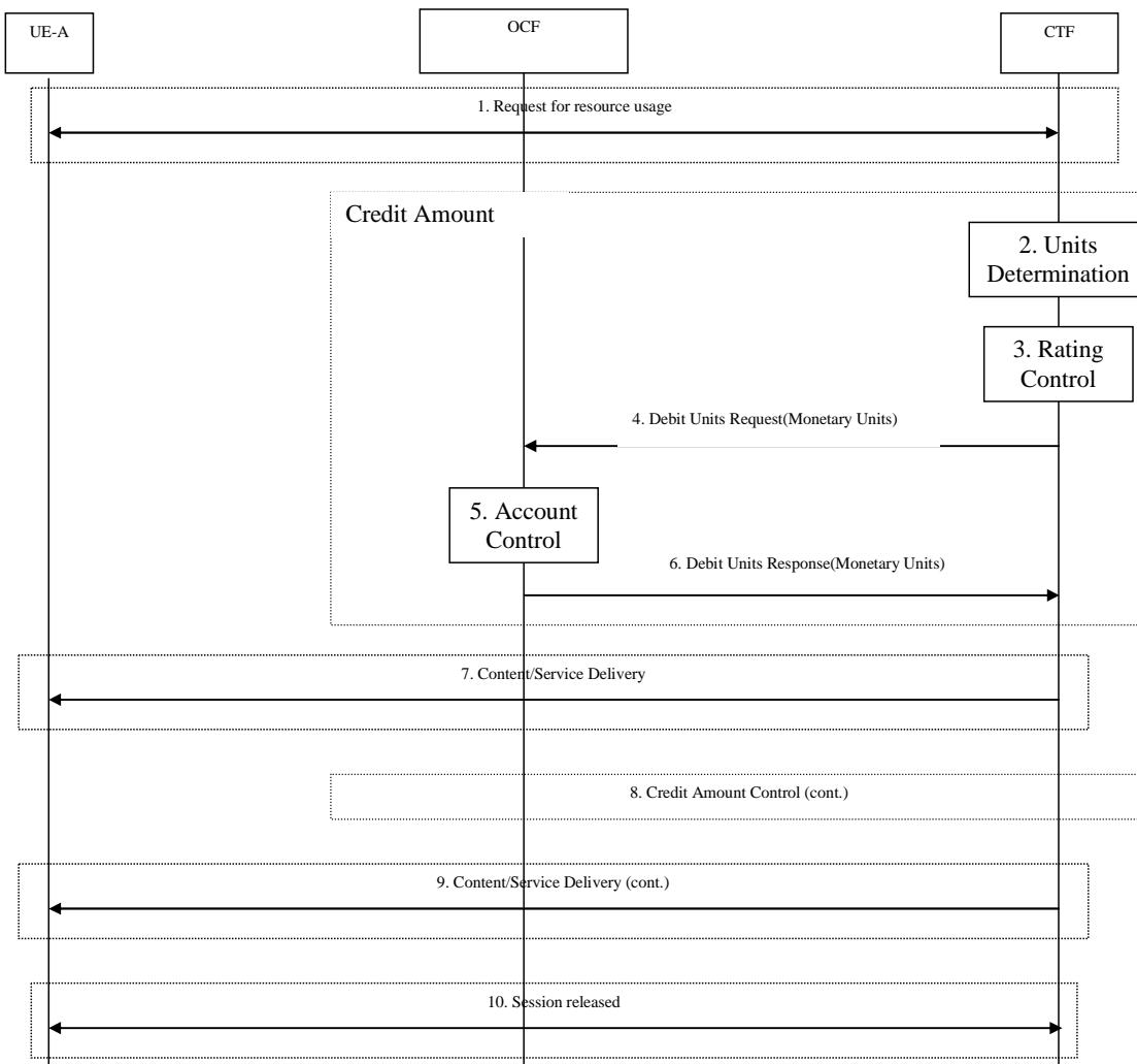
**Figure 5.2.2.1.3.1: IEC - Decentralized Rating and Decentralized Unit Determination**
