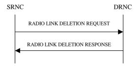
Figure: Radio Link Deletion procedure on lur, Successful Operation
