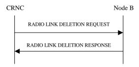
Figure: Radio Link Deletion procedure on lub, Successful Operation
