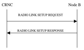
Figure: Radio Link Setup procedure on lub, Successful Operation
