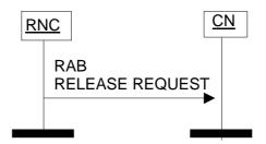
Figure: RAB Release Request procedure
