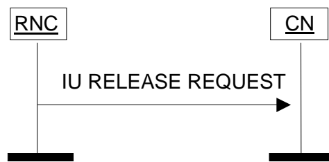
Figure: Iu Release Request procedure. Successful operation
