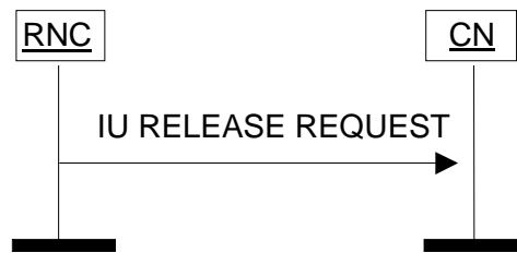
Figure: Iu Release Request procedure. Successful operation
