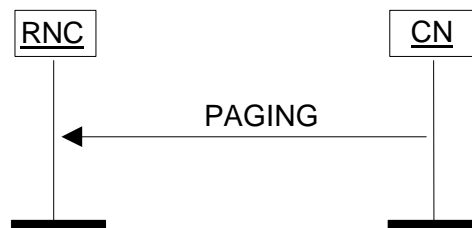
Figure: RANAP Paging procedure (Successful operation)
