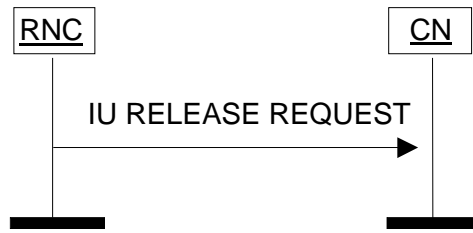
Figure: Iu Release Request procedure. Successful operation
