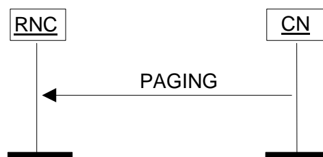
Figure: RANAP Paging procedure (Successful operation)
