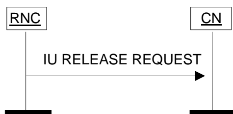
Figure: Iu Release Request procedure. Successful operation
