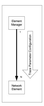
Figure 4.2.1: Architecture for Management Based Activation/Deactivation
