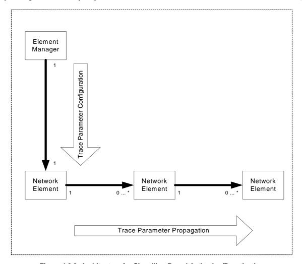
Figure 4.2.2: Architecture for Signalling Based Activation/Deactivation
