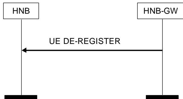
Figure 4 UE De-Register Procedure: HNB-GW Originated Successful Operation
