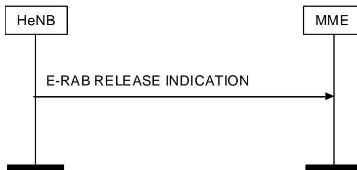
Figure 9 E-RAB Release INDICATION procedure. Successful operation
