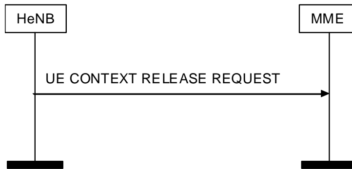
Figure 7 UE Context Release Request procedure. Successful operation
