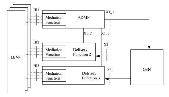
Figure 1b: Packet Switched Intercept configuration
