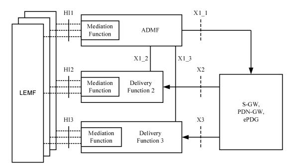
Figure 12.1.3: S-GW, PDN-GW, ePDG Intercept configuration
