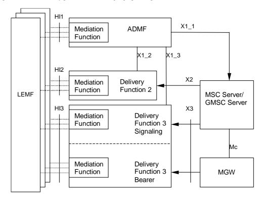
Figure 1a: Circuit switched intercept configuration
