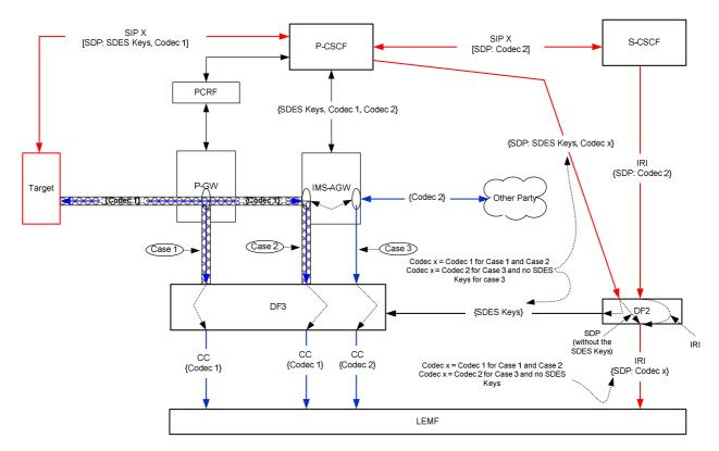
Figure G.3-1: Transcoded Media with e2ae encryption
