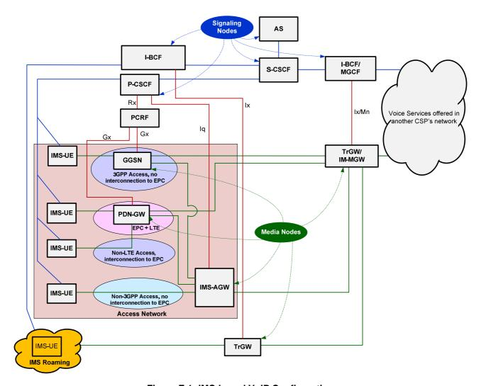
Figure E.1: IMS-based VoIP Configuration
