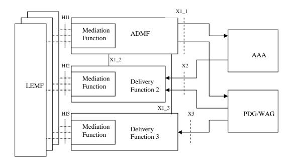
Figure 1e: WLAN Interworking Intercept configuration
