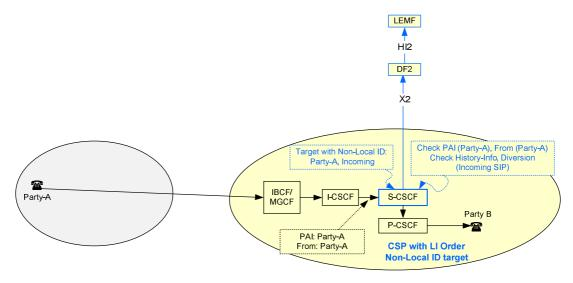
Figure I.4: IRI ICE at S-CSCF - interception of a target with Non-Local ID for incoming calls
