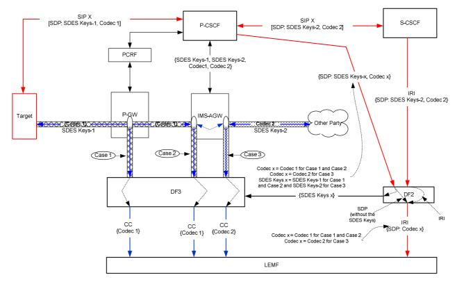
Figure G.4-1: Transcoded Media with e2e encryption
