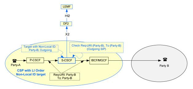
Figure I.1: IRI ICE at S-CSCF - interception of a target with Non-Local ID for outgoing calls
