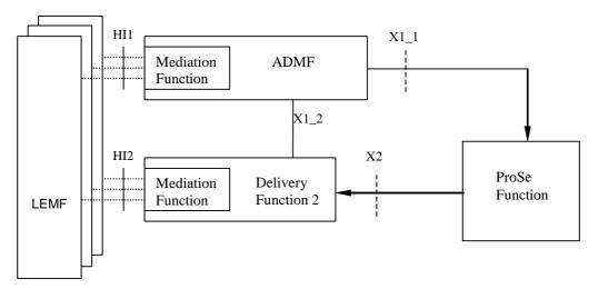
Figure 17.1-1: ProSe Direct Discovery Intercept configuration
