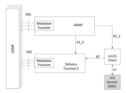
Figure 19.2.1: LALS Model for Target Positioning
