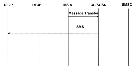
Figure B.10b: MO-SMS interception after 3G SGSN receives SMS from MS(A)
