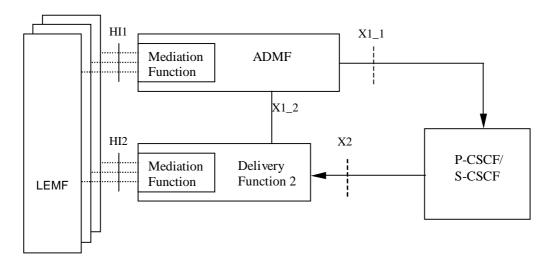
Figure 1d: IMS-CSCF Intercept configuration
