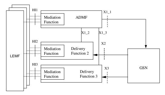
Figure 1b: Packet Switched Intercept configuration
