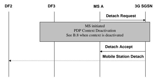
Figure B.2: Interception of mobile originated Mobile Station Detachment
