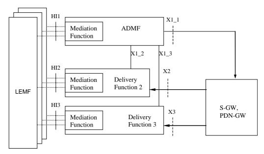
Figure 12.1.3: S-GW, PDN-GW Intercept configuration
