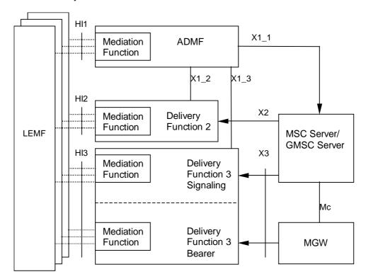
Figure 1a: Circuit switched intercept configuration
