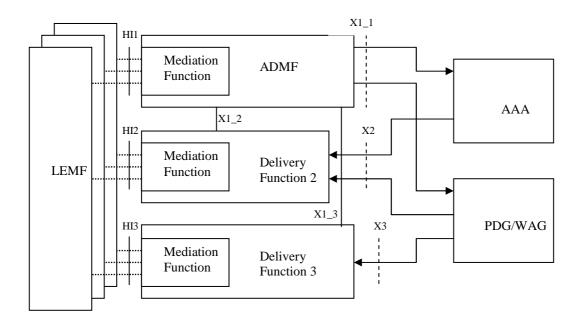
Figure 1e: WLAN Interworking Intercept configuration
