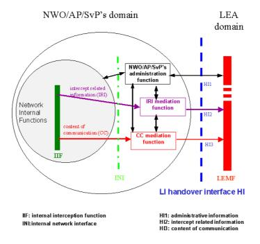
Figure 4.1: Functional block diagram showing handover interface HI
