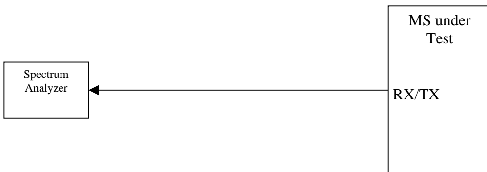
Figure A.8: Connection for Spurious Emission Test
