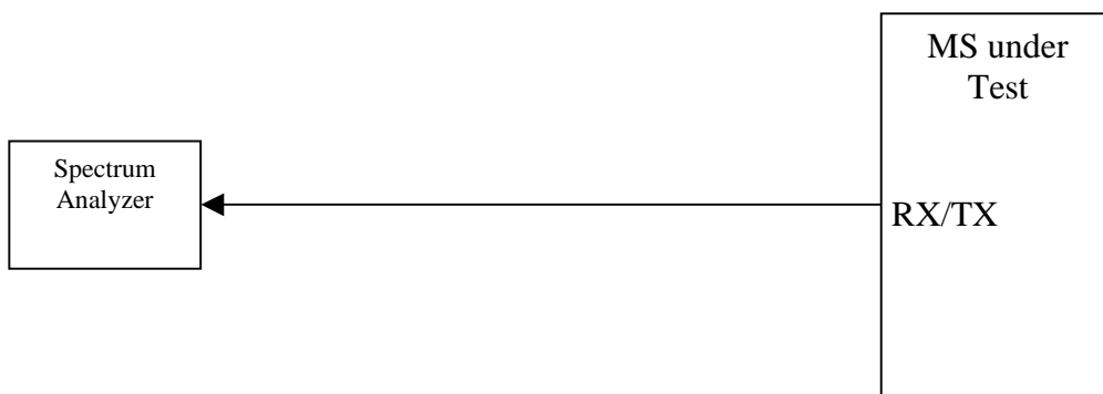
Figure A.8: Connection for Spurious Emission Test
