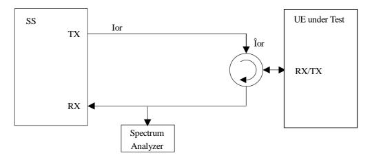
Figure A.8: Connection for Spurious Emission Test
