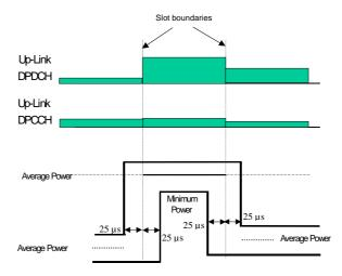
Figure 5.6.1: Transmit template during TFC change
