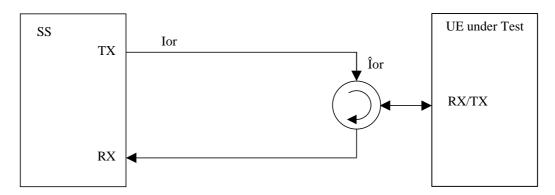
Figure A.3: Connection for Basic RX Test
