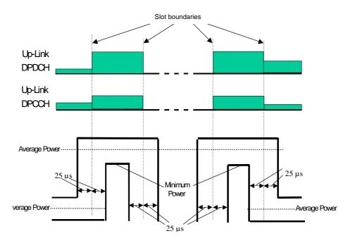
Figure 5.7.1: Transmit template during Compressed mode
