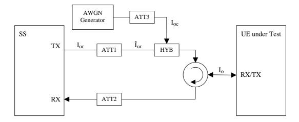
**Figure A.9: Connection for Static Propagation Test**
