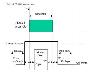
Figure 5.5.1: Transmit ON/OFF template for PRACH preambles
