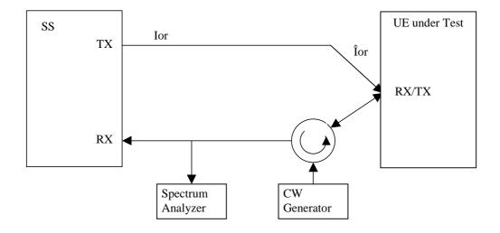
Figure A.2: Connection for TX Intermodulation Test
