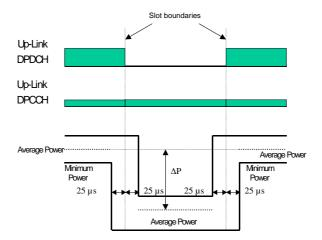
Figure 5.6.2: Transmit template during DTX
