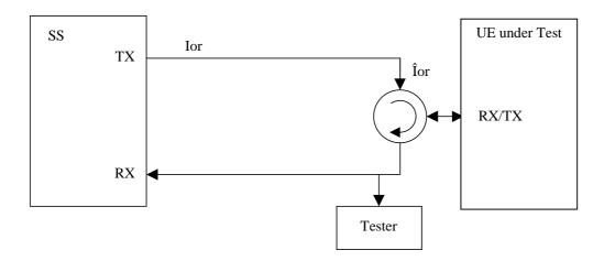
Figure A.1: Connection for Basic TX Test
