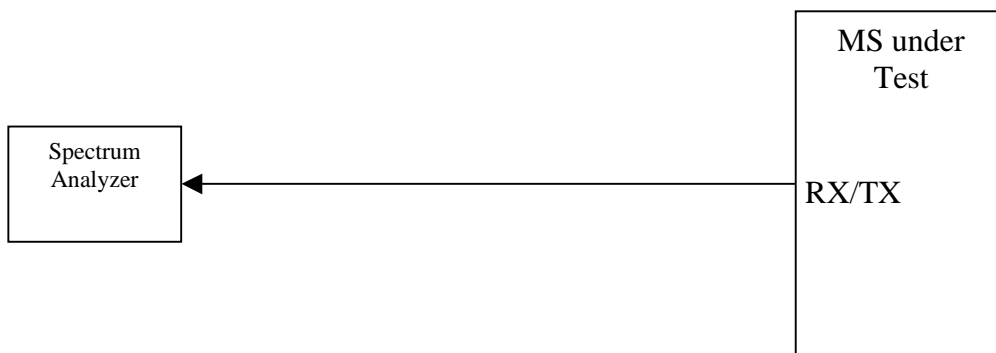
Figure A.8: Connection for Spurious Emission Test
