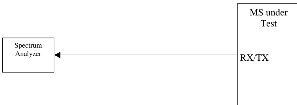
Figure A.8: Connection for Spurious Emission Test
