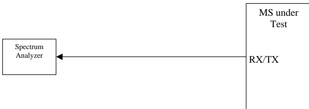
Figure A.8: Connection for Spurious Emission Test
