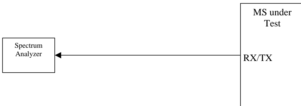
Figure A.8: Connection for Spurious Emission Test
