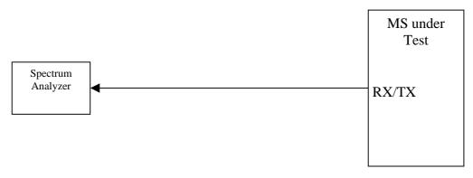
Figure A.8: Connection for Spurious Emission Test
