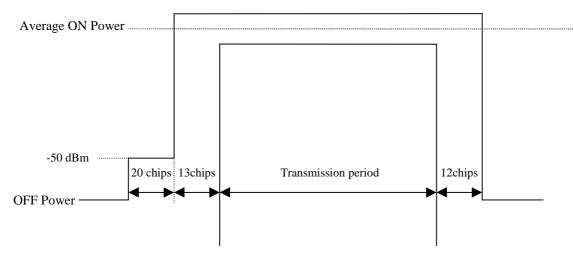
Figure 5.4.4.2.2: Transmit ON/OFF template for 1,28Mcps TDD Option
