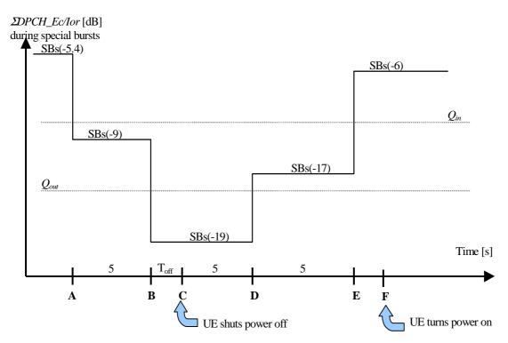
Figure 5.4.6.2.2: Conditions for out-of-synch handling in the UE. The indicated thresholds Q<sub>out</sub> andQ<sub>in</sub> are only informative. Conditions apply for 1,28 Mcps TDD Option– discontinuous transmission
