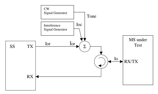
Figure A.7: Connection for RX Test with both Interference and additional CW
