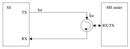
Figure A.3: Connection for Basic RX Test
