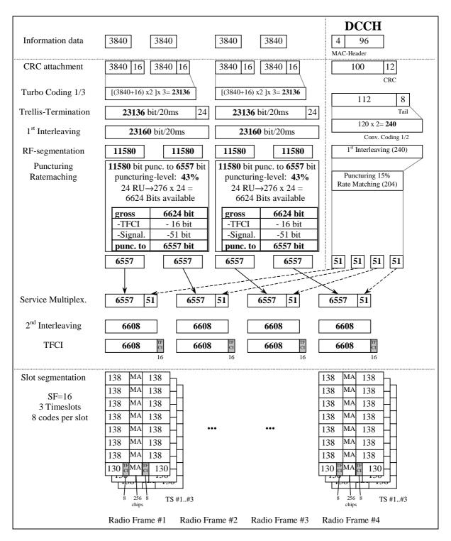
C.3.4.2 DL reference measurement channel (384 kbps) for 1,28 Mcps TDD Option
