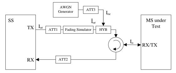
Figure A.10: Connection for Multiple Fading Channel Test
