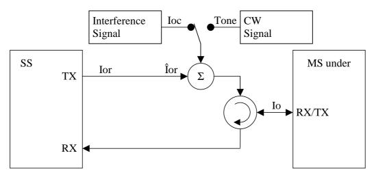
Figure A.5: Connection for RX Test with Interference or additional CW
