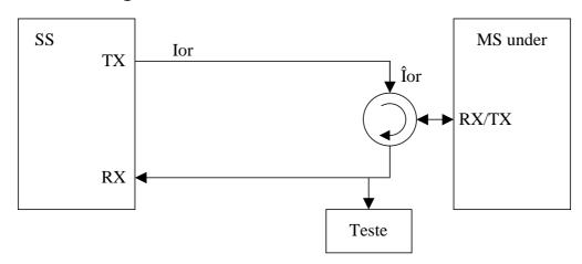
Figure A.1: Connection for Basic TX Test
