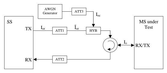
Figure A.9: Connection for Static Channel Test
