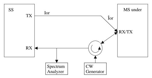
Figure A.2: Connection for TX Intermodulation Test
