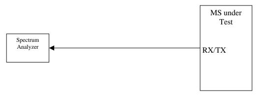
Figure A.8: Connection for Spurious Emission Test
