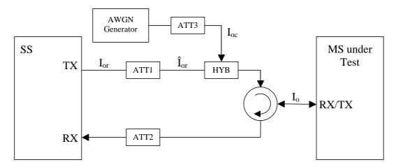
Figure A.9: Connection for Static Channel Test
