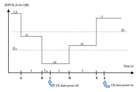
Figure 5.4.5.2.2: Conditions for out-of-synch handling in the UE. The indicated thresholds Q<sub>out</sub> andQ<sub>in</sub> are only informative. Conditions apply for 1,28 Mcps TDD Option – continuous transmission
