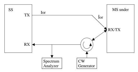
Figure A.2: Connection for TX Intermodulation Test
