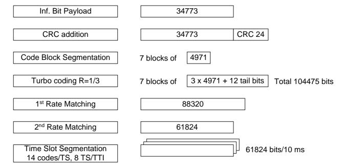
Figure C.4.1.4: Coding for HS-PDSCH fixed reference channel with 16-QAM modulation for the VA120 Channel – Category 8
