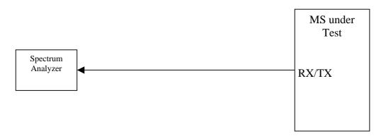
**Figure A.8: Connection for Spurious Emission Test**
