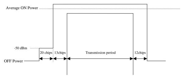
Figure 5.4.4.2.2: Transmit ON/OFF template for 1,28Mcps TDD Option
