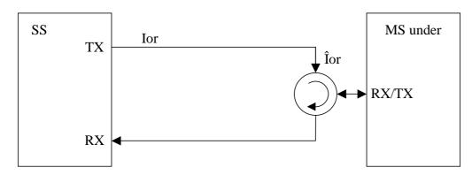
Figure A.3: Connection for Basic RX Test
