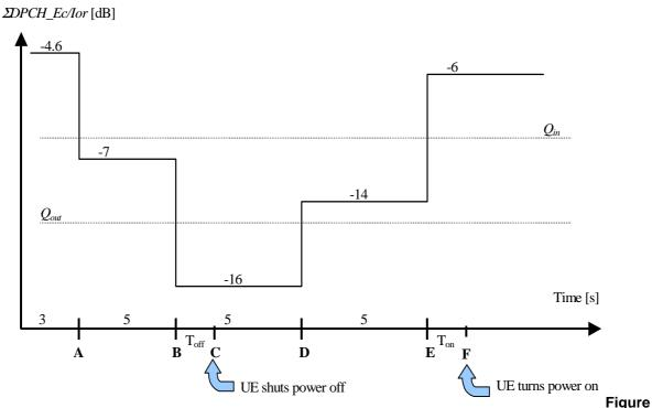
5.4.5.2.1: Test case for out-of-synch handling in the UE. Conditions apply for 3,84 Mcps TDD Option – continuous transmission
