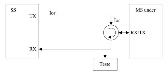
Figure A.1: Connection for Basic TX Test
