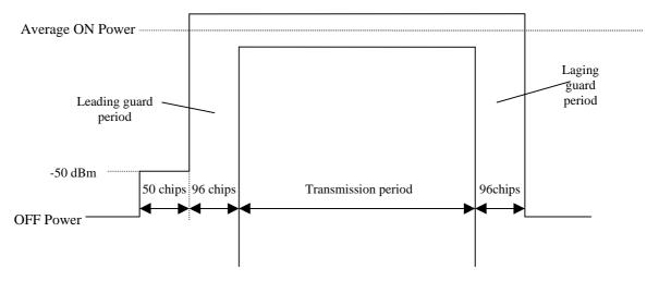
Figure 5.4.4.2.1: Transmit ON/OFF template for 3,84 Mcps TDD Option
