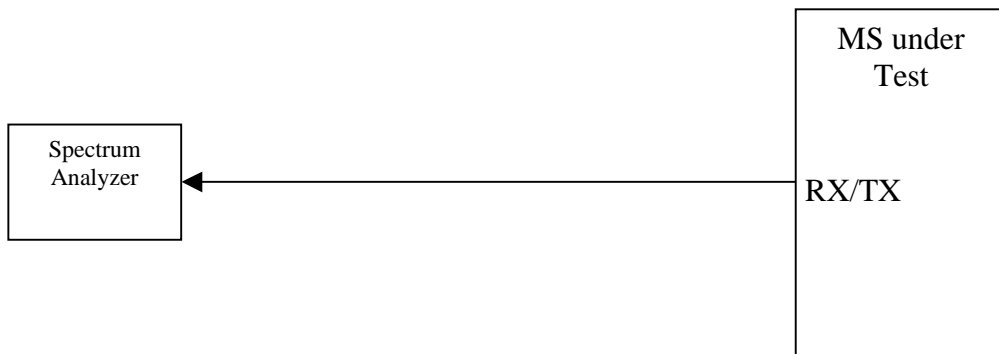
Figure A.8: Connection for Spurious Emission Test
