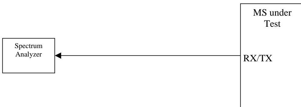
Figure A.8: Connection for Spurious Emission Test
