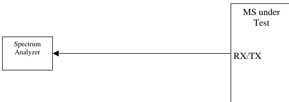
Figure A.8: Connection for Spurious Emission Test
