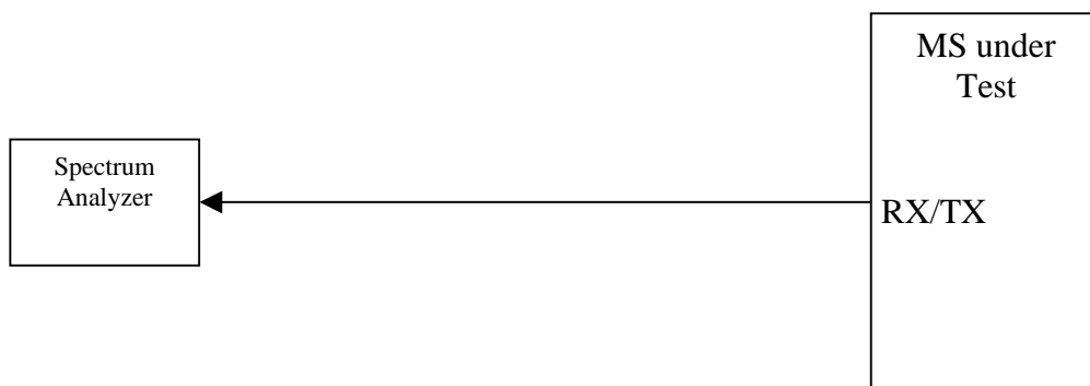
Figure A.8: Connection for Spurious Emission Test
