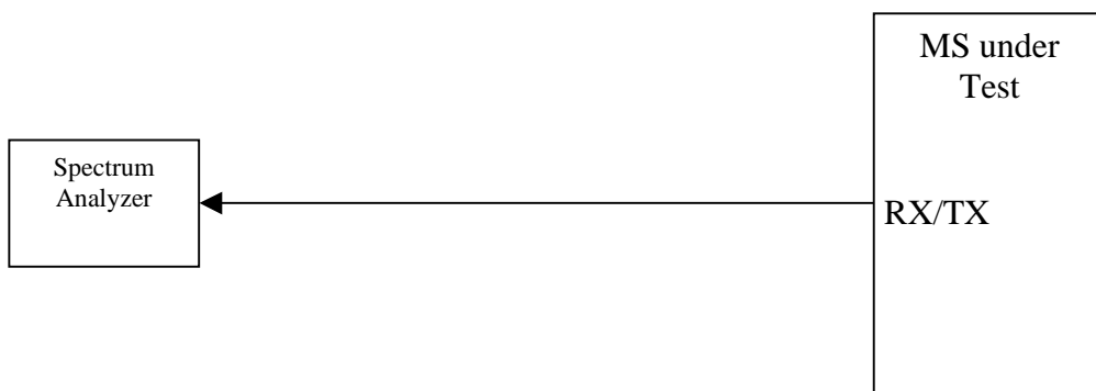
Figure A.8: Connection for Spurious Emission Test
