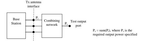
Figure 4.5.7.2-1: Transmitter test set-up
