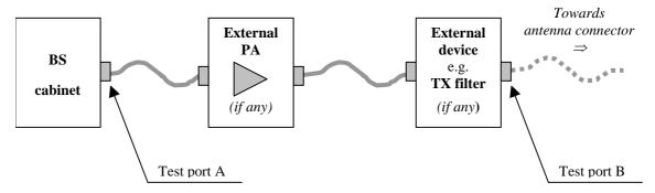
Figure 4.5-1: Transmitter test ports
