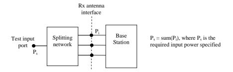
Figure 4.5.7.1-1: Receiver test set-up
