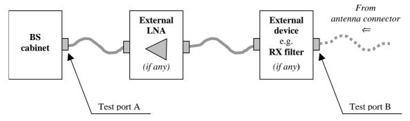
Figure 4.5-2: Receiver test ports
