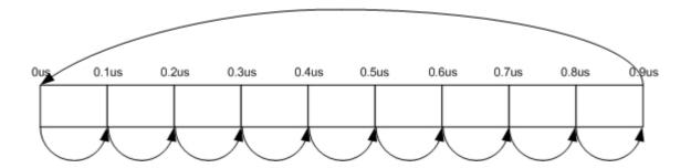
Figure 8.4.1.4.2-2: Timing offset scheme
