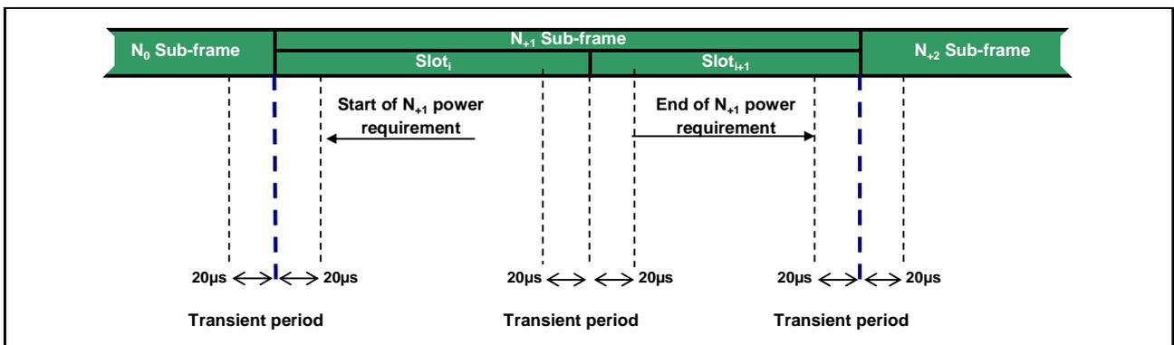
Figure 6.3.4.3-1: Transmission power template
