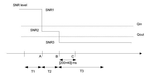
Figure A.7.3.18.1-1 SNR variation for out-of-sync testing
