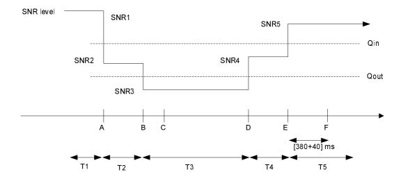
Figure A.7.3.2.1-1 SNR variation for in-sync testing
