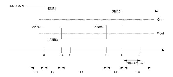
Figure A.7.3.4.1-1. SNR variation for in-sync testing
