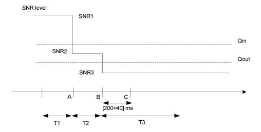
Figure A.7.3.9.1-1 SNR variation for out-of-sync testing
