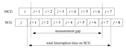
(b) measurement GAP for asynchronous dual connectivity
