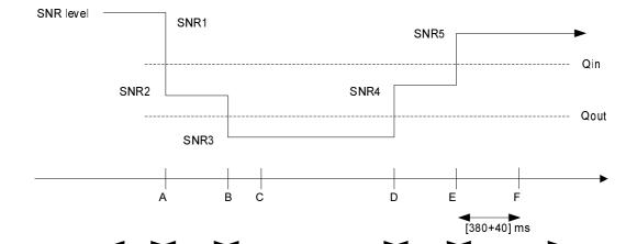
Figure A.7.3.31.1-1: SNR variation for in-sync testing
