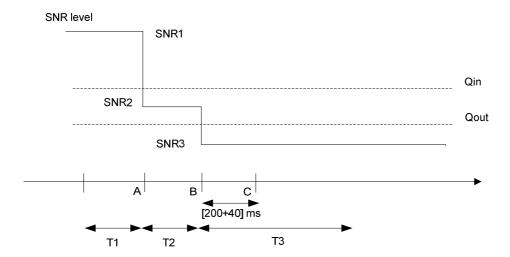
Figure A.7.3.3.1-1. SNR variation for out-of-sync testing
