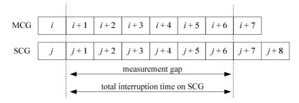
(a) measurement GAP for synchronous dual connectivity
