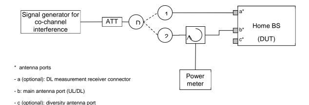
Figure I.1-5: (Option 1) Measuring system set-up for Home BS output power for co-channel E-UTRA protection
