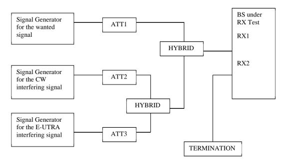
Figure I.2-7: Measuring system Set-up for intermodulation characteristics
