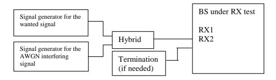
Figure I.2-2: Measuring system Set-up for Dynamic range
