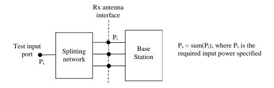
Figure 4.5.7.1-1: Receiver test set-up
