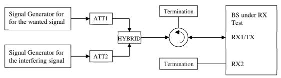
Figure I.2-5: Measuring system Set-up for Blocking characteristics
