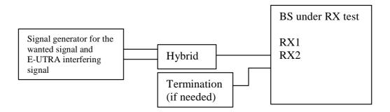
Figure I.2-3: Measuring system Set-up for In-channel selectivity
