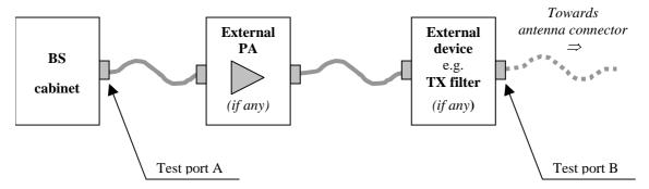
Figure 4.5-1: Transmitter test ports
