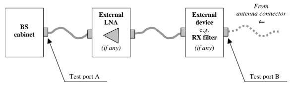
Figure 4.5-2: Receiver test ports
