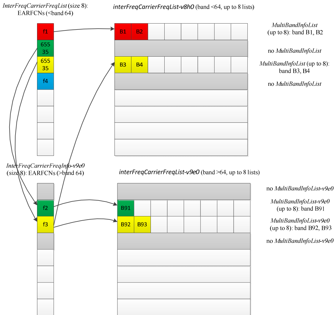
Figure D.1.2-1: Mapping of EARFCNs to MultiBandInfoList/MultiBandInfoList-v9e0
