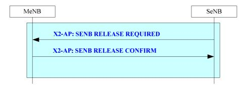
Figure 20.2.2.2f-1: SeNB initiated SeNB Release procedure
