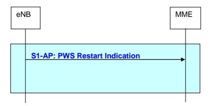
Figure 19.2.2.22-1: PWS Restart Indication procedure
