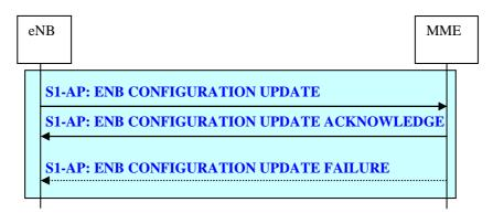
Figure 19.2.2.9-1: eNB Configuration Update procedure
