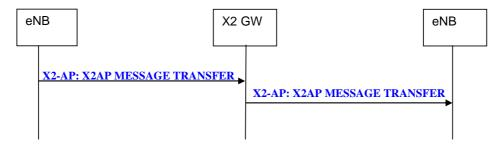
Figure 20.2.2.17-1: X2AP Message Transfer procedure
