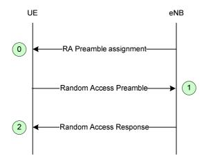
Figure 10.1.5.2-1: Non-contention based Random Access Procedure
