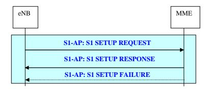
Figure 19.2.2.8-1: S1 Setup procedure
