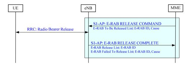
Figure 19.2.2.4.3-1: E-RAB Release procedure
