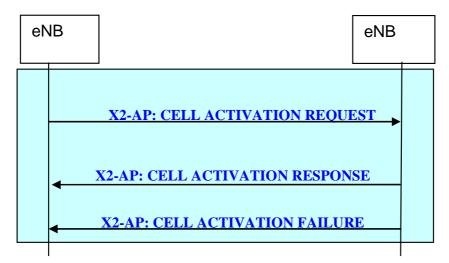
Figure 20.2.2.15-1: Cell Activation procedure
