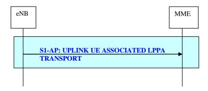
Figure 19.2.2.18.2-1: Uplink UE Associated LPPa Transport procedure
