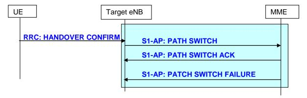
Figure 19.2.2.5.5-1: Path Switch procedure
