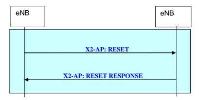
Figure 20.2.2.9-1: Reset procedure
