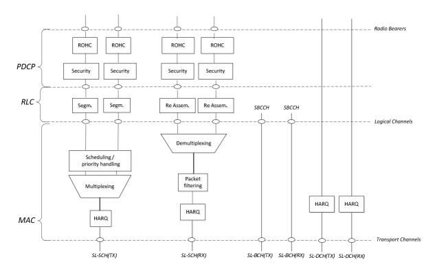
Figure 6-3: Layer 2 Structure for Sidelink
