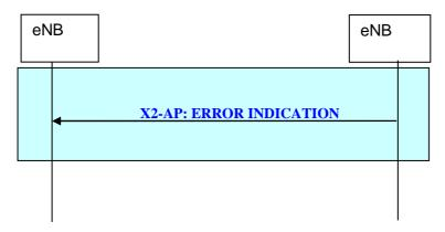
Figure 20.2.2.5-1: Error Indication procedure
