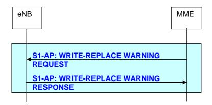
Figure 19.2.2.13.1-1: Write-Replace Warning procedure
