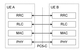
Figure 23.10.2.2-1: Control-Plane protocol stack for sidelink communication
