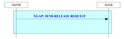
Figure 20.2.2.2e-1: MeNB initiated SeNB Release procedure
