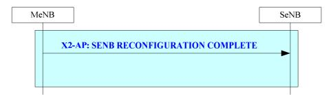
Figure 20.2.2.2b-1: SeNB Reconfiguration Completion procedure
