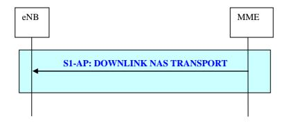
Figure 19.2.2.6-3: Downlink NAS Transport procedure
