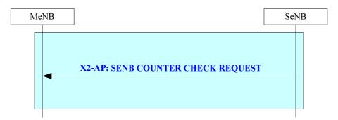
Figure 20.2.2.2g-1: SeNB Counter Check procedure
