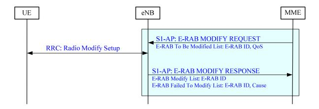
Figure 19.2.2.4.2-1: E-RAB Modification procedure
