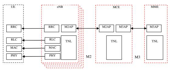
Figure 15.1.3-1: The E-MBMS c-plane architecture
