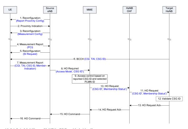
Figure 10.5.1.2-1: Mobility to HeNB"s CSG and hybrid cells.
