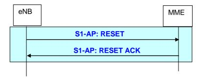
Figure 19.2.2.7.1a-1: eNB initiated Reset procedure
