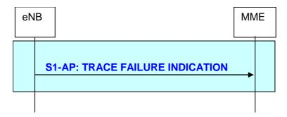
Figure 19.2.2.19.2-1: Trace Failure Indication procedure
