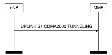
Figure 19.2.2.16.2-1: Uplink S1 CDMA2000 Tunnelling procedure
