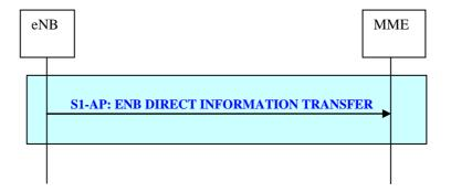
Figure 19.2.2.14-1: eNB Direct Information Transfer procedure
