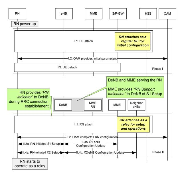
Figure 4.7.6.3-1: RN startup procedure
