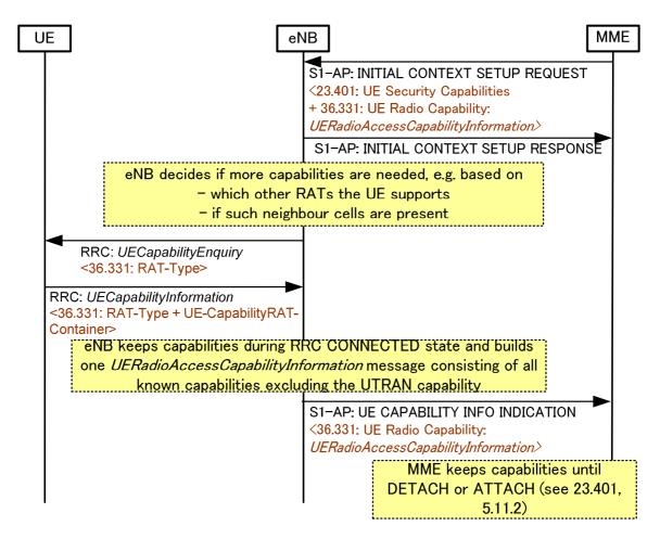
Figure 18-1: Initial UE Capability Handling
