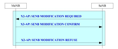
Figure 20.2.2.2d-1: SeNB initiated SeNB Modification procedure
