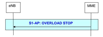
Figure 19.2.2.12.2-1: Overload Stop procedure
