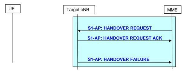
Figure 19.2.2.5.2-1: Handover resource allocation procedure
