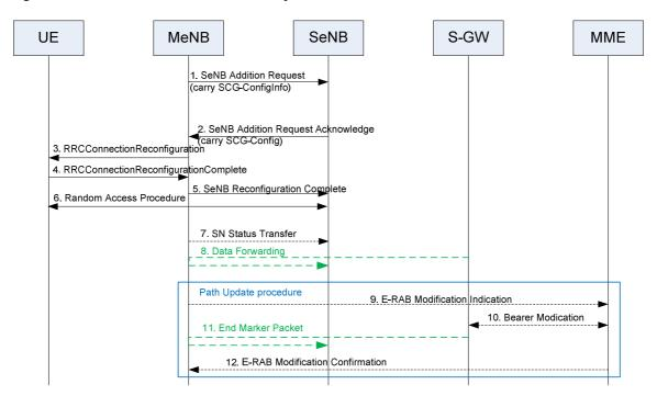
Figure 10.1.2.8.1-1: SeNB Addition procedure
