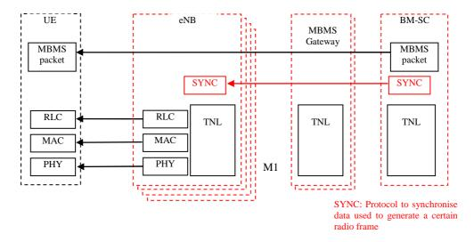
Figure 15.1.2-1: The overall u-plane architecture of the MBMS content synchronization
