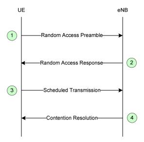
Figure 10.1.5.1-1: Contention based Random Access Procedure
