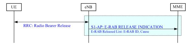
Figure 19.2.2.4.4-1: E-RAB Release Indication procedure
