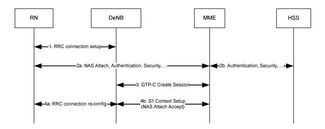
Figure 4.7.6.1-1: RN attach procedure
