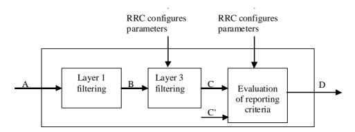
Figure 10.6-1: Measurement model
