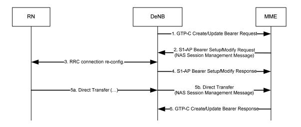
Figure 4.7.6.2-1: DeNB-initiated bearer activation/modification procedure
