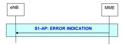
Figure 19.2.2.7.2b-1: MME initiated Error Indication procedure
