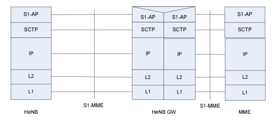
Figure 4.6.3.2-2: Control plane for S1-MME Interface for HeNB to MME with the HeNB GW  $\,$
