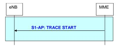
Figure 19.2.2.19.1-1: Trace Start procedure
