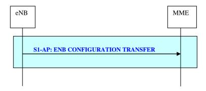
Figure 19.2.2.9a-1: eNB Configuration Transfer procedure
