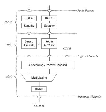
Figure 6-2: Layer 2 Structure for UL
