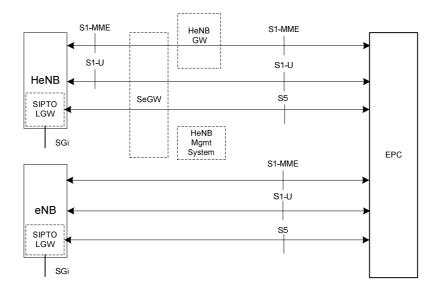
Figure 4.8.2-1: E-UTRAN - SIPTO@LN with collocated L-GW - Logical Architecture
