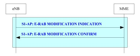
Figure 19.2.2.4.5-1: E-RAB Modification Indication procedure
