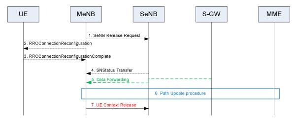
Figure 10.1.2.8.3-1: SeNB Release procedure – MeNB initiated
