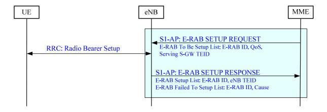
Figure 19.2.2.4.1-1: E-RAB Setup procedure
