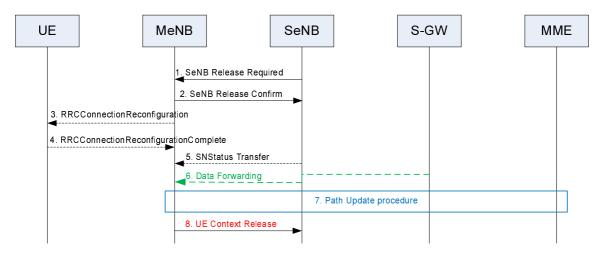
Figure 10.1.2.8.3-2: SeNB Release procedure – SeNB initiated
