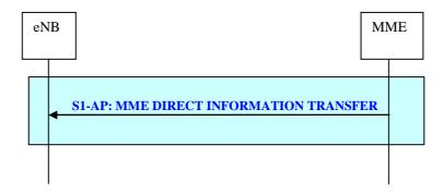
Figure 19.2.2.15-1: MME Direct Information Transfer procedure
