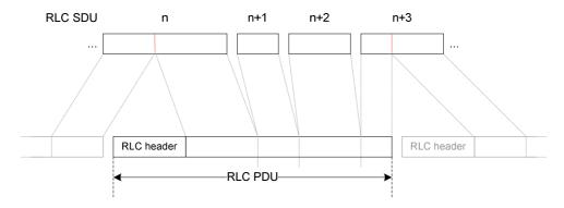
Figure 6.2.2-1: RLC PDU Structure
