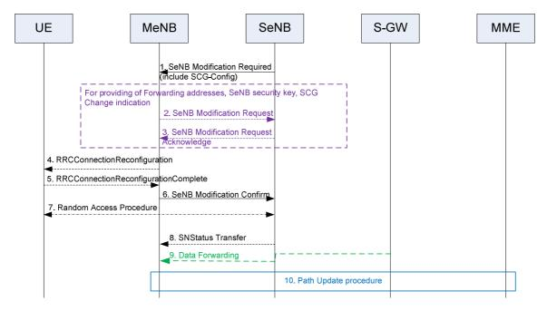
Figure 10.1.2.8.2-2: SeNB Modification procedure - SeNB initiated
