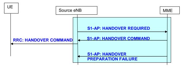
Figure 19.2.2.5.1-1: Handover preparation procedure
