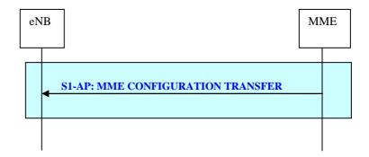
Figure 19.2.2.10a-1: MME Configuration Transfer procedure
