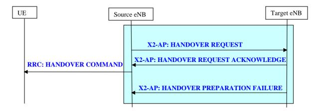
Figure 20.2.2.1-1: Handover Preparation procedure
