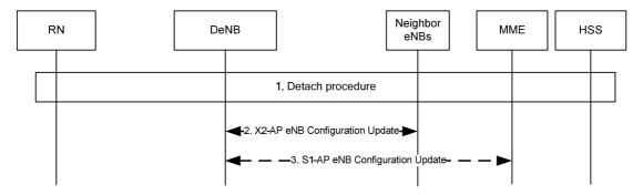
Figure 4.7.6.4-1: RN detach procedure
