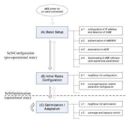
Figure 22.1-1: Ramifications of Self-Configuration /Self-Optimization functionality
