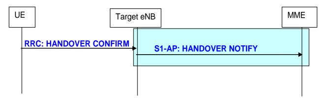
Figure 19.2.2.5.3-1: Handover completion procedure
