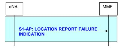
Figure 19.2.2.11.3-1: Location Report Failure Indication procedure
