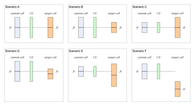
Figure 10.1.3-1: Inter and Intra-frequency measurements scenarios
