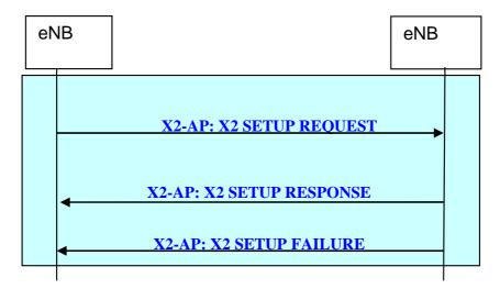
Figure 20.2.2.7-1: X2 Setup procedure
