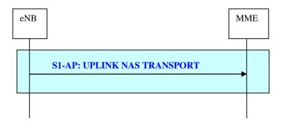
Figure 19.2.2.6-2: Uplink NAS Transport procedure
