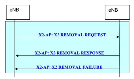
Figure 20.2.2.18-1: X2 Removal procedure
