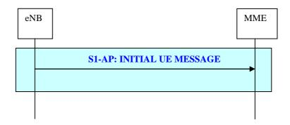
Figure 19.2.2.6-1: Initial UE Message procedure
