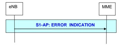
Figure 19.2.2.7.2a-1: eNB initiated Error Indication procedure
