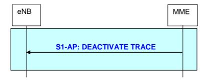
Figure 19.2.2.19.3-1: Deactivate Trace procedure
