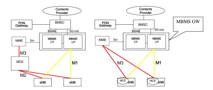
Figure 15.1.1-2: eMBMS Architecture deployment alternatives
