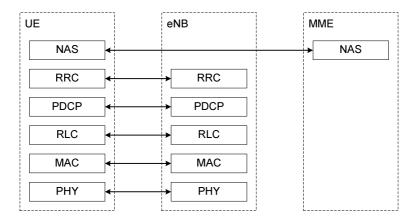
Figure 4.3.2-1: Control-plane protocol stack
