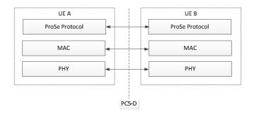
Figure 23.11.1-1: PC5 interface for sidelink discovery [62]
