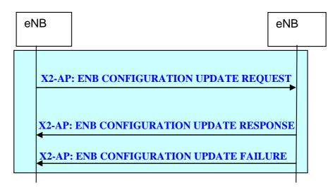
Figure 20.2.2.8-1: eNB Configuration Update procedure
