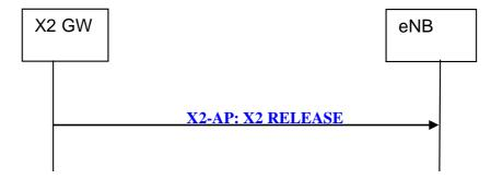
Figure 20.2.2.16-1: X2 Release procedure
