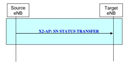
Figure 20.2.2.4-1: SN Status Transfer procedure
