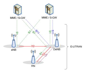
Figure 4.7.2-1: Overall E-UTRAN Architecture supporting RNs
