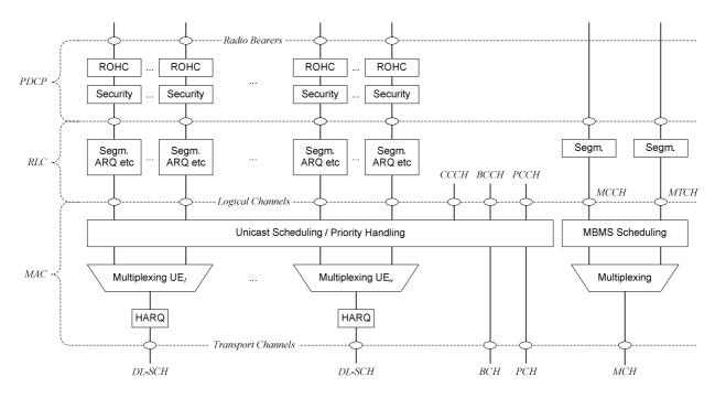
Figure 6-1: Layer 2 Structure for DL
