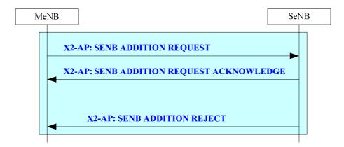
Figure 20.2.2.2a-1: SeNB Addition Preparation procedure
