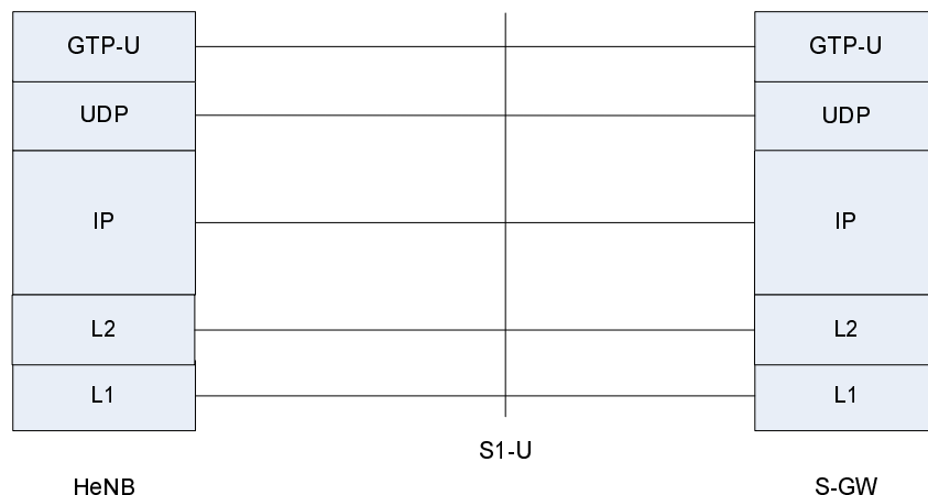
Figure 4.6.3.1-1: User plane for S1-U interface for HeNB without HeNB GW
