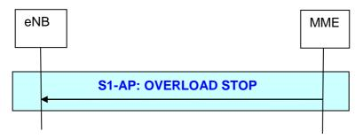
Figure 19.2.2.12.2-1: Overload Stop procedure
