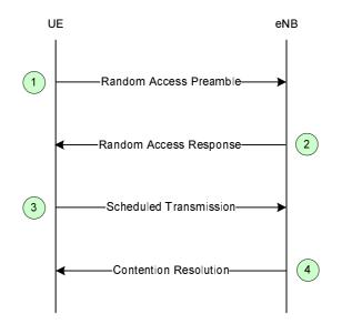
Figure 10.1.5.1-1: Contention based Random Access Procedure
