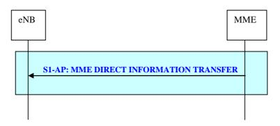
Figure 19.2.2.15-1: MME Direct Information Transfer procedure
