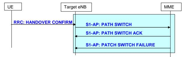
Figure 19.2.2.5.5-1: Path Switch procedure
