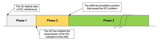
Figure 23.4.2-1: Different phases of IDC interference related operations by UE
