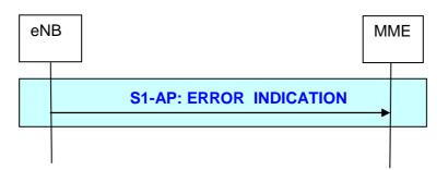
Figure 19.2.2.7.2a-1: eNB initiated Error Indication procedure
