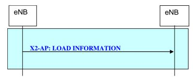
Figure 20.2.2.6-1: Load Indication procedure
