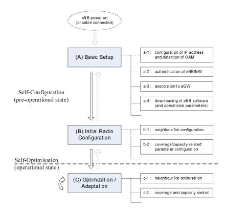
Figure 22.1-1: Ramifications of Self-Configuration /Self-Optimization functionality
