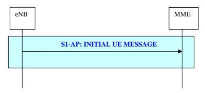
Figure 19.2.2.6-1: Initial UE Message procedure
