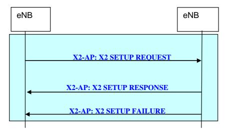
Figure 20.2.2.7-1: X2 Setup procedure
