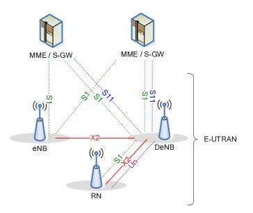
Figure 4.7.2-1: Overall E-UTRAN Architecture supporting RNs
