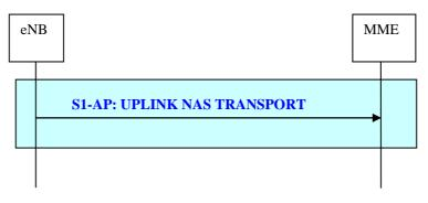
Figure 19.2.2.6-2: Uplink NAS Transport procedure
