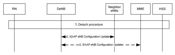
Figure 4.7.6.4-1: RN detach procedure
