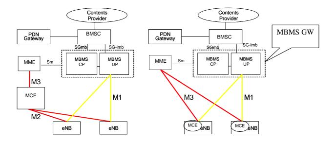
Figure 15.1.1-2: eMBMS Architecture deployment alternatives
