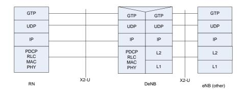
Figure 4.7.3-2: X2 user plane protocol stack for supporting RNs
