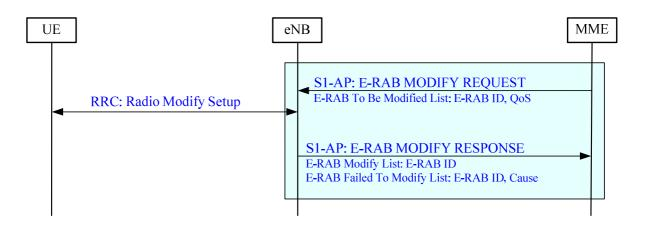
Figure 19.2.2.4.2-1: E-RAB Modification procedure
