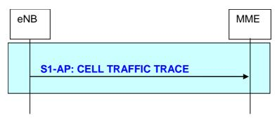
Figure 19.2.2.19.4-1: Cell Traffic Trace procedure
