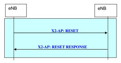
Figure 20.2.2.9-1: Reset procedure
