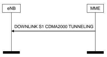
Figure 19.2.2.16.1-1: Downlink S1 CDMA2000 Tunnelling procedure
