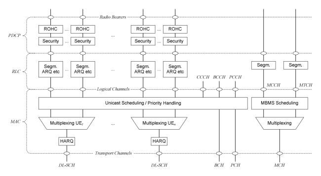
Figure 6-1: Layer 2 Structure for DL
