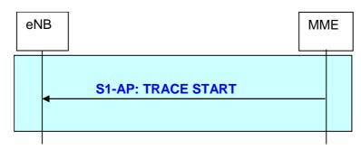
Figure 19.2.2.19.1-1: Trace Start procedure
