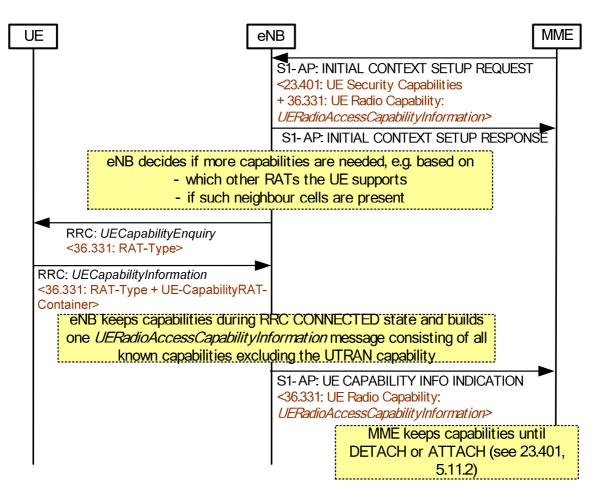
Figure 18-1: Initial UE Capability Handling
