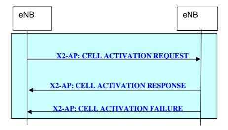
Figure 20.2.2.15-1: Cell Activation procedure
