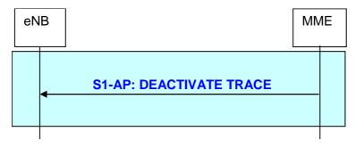
Figure 19.2.2.19.3-1: Deactivate Trace procedure
