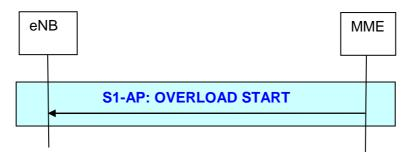
Figure 19.2.2.12.1-1 Overload Start procedure
