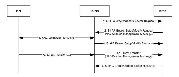
Figure 4.7.6.2-1: DeNB-initiated bearer activation/modification procedure
