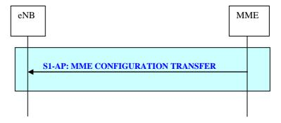
Figure 19.2.2.10a-1: MME Configuration Transfer procedure
