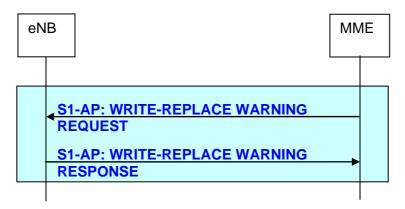
Figure 19.2.2.13.1-1: Write-Replace Warning procedure
