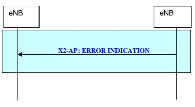
Figure 20.2.2.5-1: Error Indication procedure
