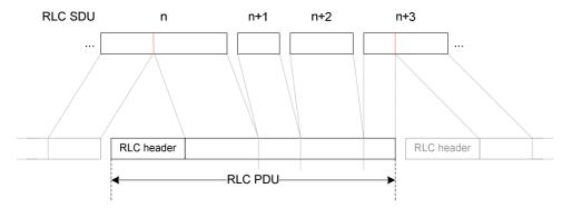
Figure 6.2.2-1: RLC PDU Structure
