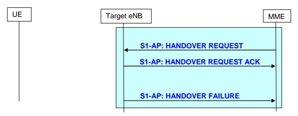
Figure 19.2.2.5.2-1: Handover resource allocation procedure
