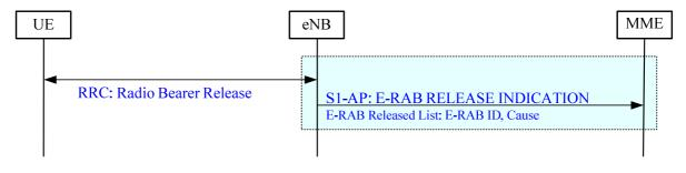
Figure 19.2.2.4.4-1: E-RAB Release Indication procedure
