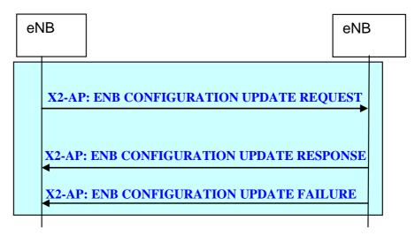
Figure 20.2.2.8-1: eNB Configuration Update procedure
