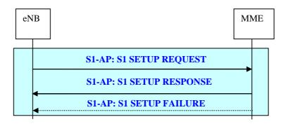
Figure 19.2.2.8-1: S1 Setup procedure
