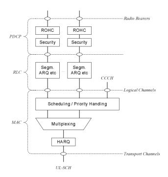
Figure 6-2: Layer 2 Structure for UL
