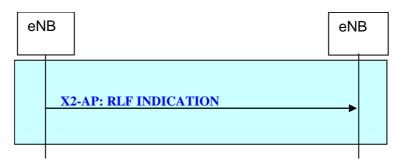
Figure 20.2.2.12-1: Radio Link Failure Indication procedure
