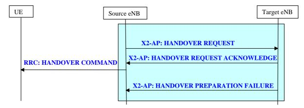
Figure 20.2.2.1-1: Handover Preparation procedure
