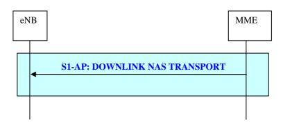
Figure 19.2.2.6-3: Downlink NAS Transport procedure
