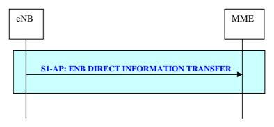
Figure 19.2.2.14-1: eNB Direct Information Transfer procedure
