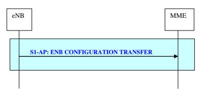
Figure 19.2.2.9a-1: eNB Configuration Transfer procedure
