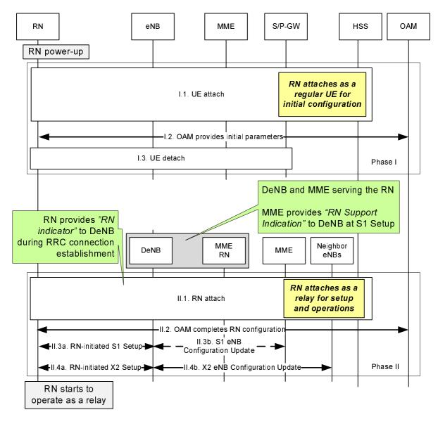
Figure 4.7.6.3-1: RN startup procedure
