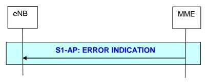
Figure 19.2.2.7.2b-1: MME initiated Error Indication procedure
