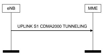
Figure 19.2.2.16.2-1: Uplink S1 CDMA2000 Tunnelling procedure
