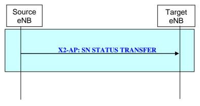
Figure 20.2.2.4-1: SN Status Transfer procedure
