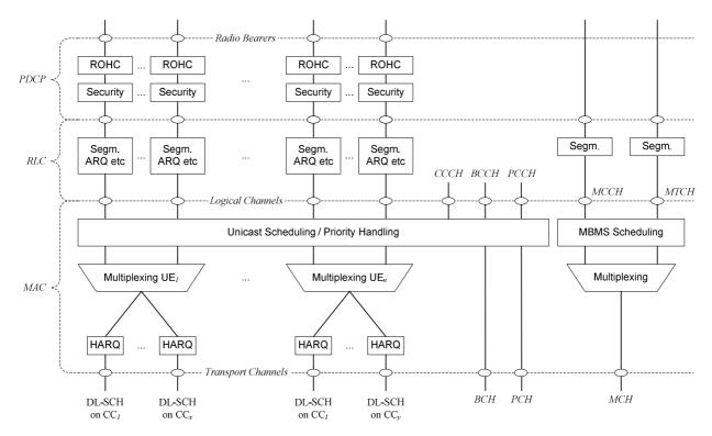
Figure 6.4-1: Layer 2 Structure for DL with CA configured
