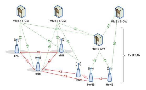
Figure 4.6.1-2: Overall E-UTRAN Architecture with deployed HeNB GW.
