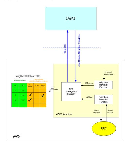
Figure 22.3.2a-1: Interaction between eNB and O&M due to ANR
