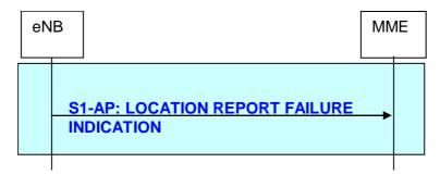
Figure 19.2.2.11.3-1: Location Report Failure Indication procedure
