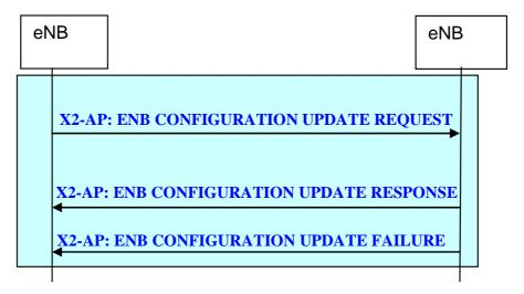
Figure 20.2.2.8-1: eNB Configuration Update procedure
