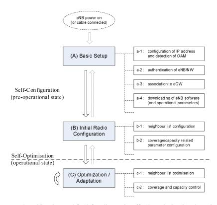
Figure 22.1-1: Ramifications of Self-Configuration /Self-Optimization functionality
