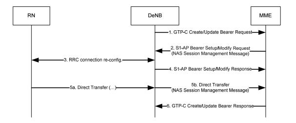
Figure 4.7.6.2-1: DeNB-initiated bearer activation/modification procedure
