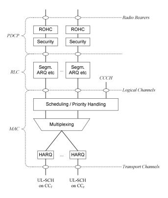
Figure 6.4-2: Layer 2 Structure for UL with CA configured
