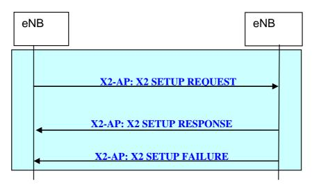
Figure 20.2.2.7-1: X2 Setup procedure
