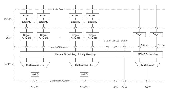
Figure 6-1: Layer 2 Structure for DL
