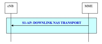
Figure 19.2.2.6-3: Downlink NAS Transport procedure
