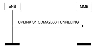
Figure 19.2.2.16.2-1: Uplink S1 CDMA2000 Tunnelling procedure
