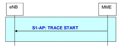
Figure 19.2.2.19.1-1: Trace Start procedure
