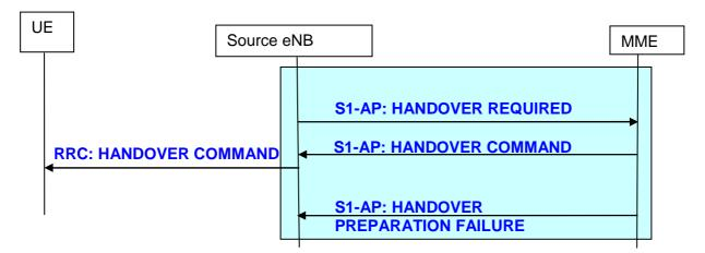
Figure 19.2.2.5.1-1: Handover preparation procedure
