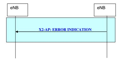
Figure 20.2.2.5-1: Error Indication procedure
