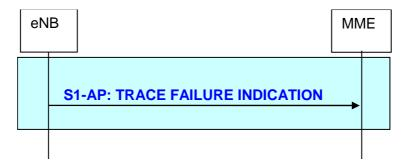
Figure 19.2.2.19.2-1: Trace Failure Indication procedure
