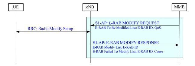
Figure 19.2.2.4.2-1: E-RAB Modification procedure
