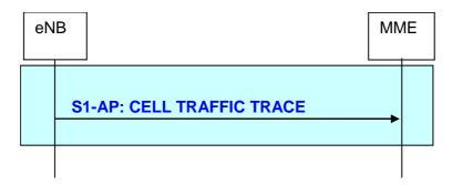
Figure 19.2.2.19.4-1: Cell Traffic Trace procedure
