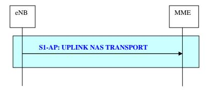
Figure 19.2.2.6-2: Uplink NAS Transport procedure
