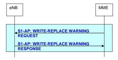
Figure 19.2.2.13.1-1: Write-Replace Warning procedure
