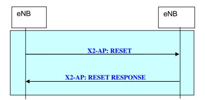
Figure 20.2.2.9-1: Reset procedure
