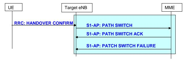
Figure 19.2.2.5.5-1: Path Switch procedure
