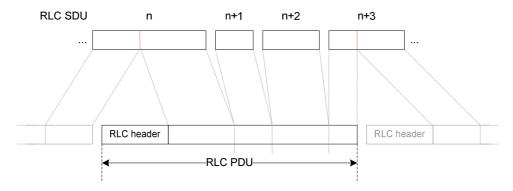
Figure 6.2.2-1: RLC PDU Structure
