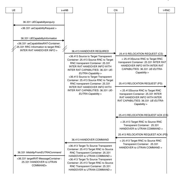
Figure 19.2.2.5.6-7. Handover of PS and CS domain service from EUTRAN to UTRAN, normal flow
