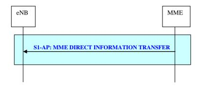
Figure 19.2.2.15-1: MME Direct Information Transfer procedure
