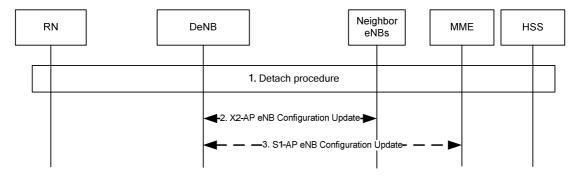
Figure 4.7.6.4-1: RN detach procedure
