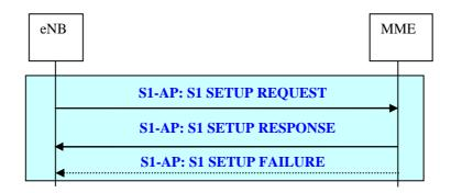
Figure 19.2.2.8-1: S1 Setup procedure
