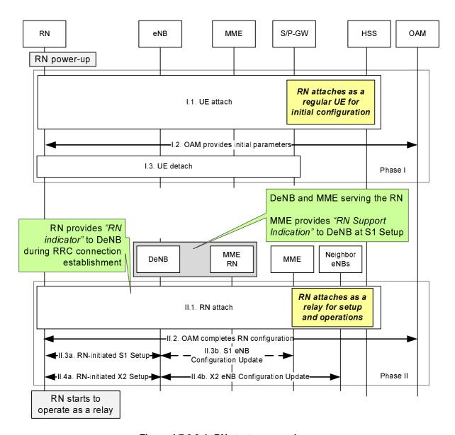
Figure 4.7.6.3-1: RN startup procedure
