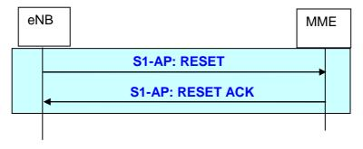
Figure 19.2.2.7.1a-1: eNB initiated Reset procedure
