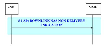
Figure 19.2.2.6-4: Downlink NAS Non Delivery Indication procedure
