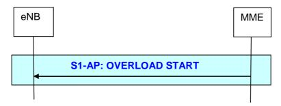
Figure 19.2.2.12.1-1 Overload Start procedure
