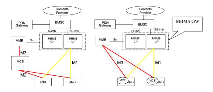
Figure 15.1.1-2: eMBMS Architecture deployment alternatives
