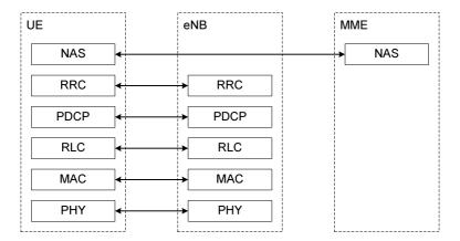
Figure 4.3.2-1: Control-plane protocol stack
