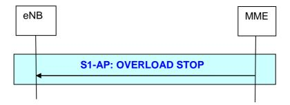
Figure 19.2.2.12.2-1: Overload Stop procedure
