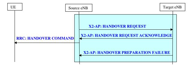
Figure 20.2.2.1-1: Handover Preparation procedure
