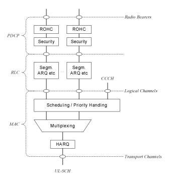
Figure 6-2: Layer 2 Structure for UL
