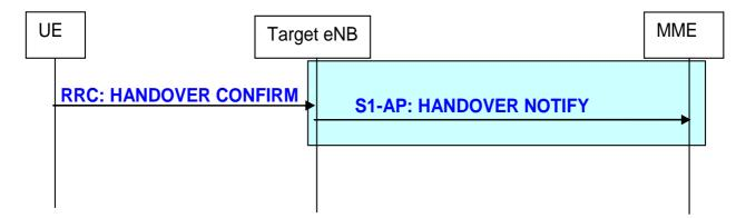
Figure 19.2.2.5.3-1: Handover completion procedure
