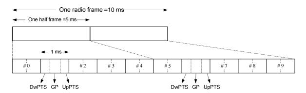
Figure 5.1-2: Frame structure type 2 (for 5ms switch-point periodicity)
