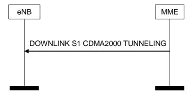
Figure 19.2.2.16.1-1: Downlink S1 CDMA2000 Tunnelling procedure
