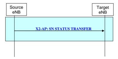
Figure 20.2.2.4-1: SN Status Transfer procedure
