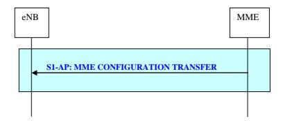
Figure 19.2.2.10a-1: MME Configuration Transfer procedure
