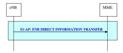
Figure 19.2.2.14-1: eNB Direct Information Transfer procedure
