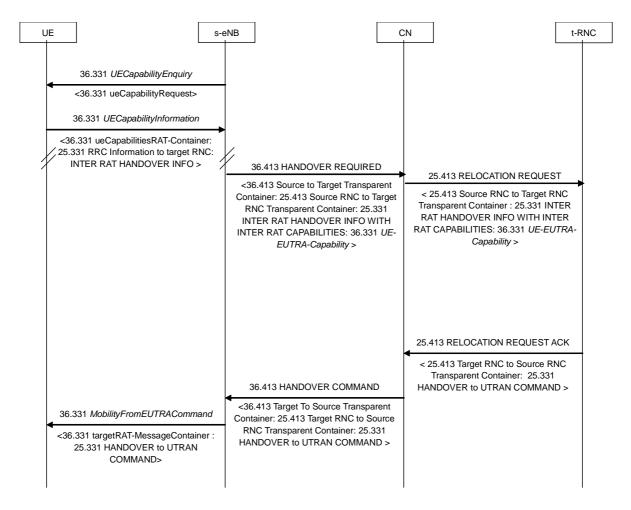
Figure 19.2.2.5.6-6. Handover of PS or CS domain service from EUTRAN to UTRAN, normal flow
