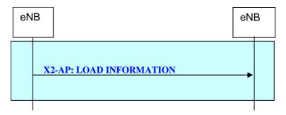
Figure 20.2.2.6-1: Load Indication procedure
