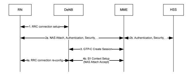
Figure 4.7.6.1-1: RN attach procedure
