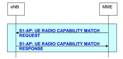
Figure 19.2.2.21-1: UE Radio Capability Match procedure
