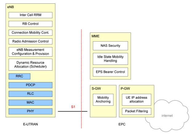
Figure 4.1-1: Functional Split between E-UTRAN and EPC
