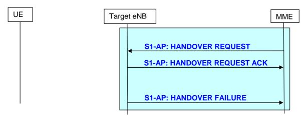
Figure 19.2.2.5.2-1: Handover resource allocation procedure
