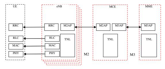
Figure 15.1.3-1: The E-MBMS c-plane architecture
