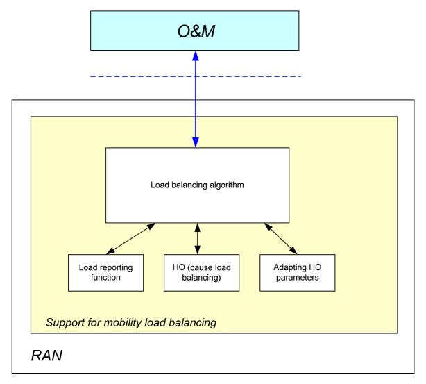
Figure 22.4.1.1-1: Functional architecture of SON load balancing
