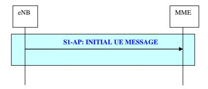
Figure 19.2.2.6-1: Initial UE Message procedure
