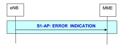
Figure 19.2.2.7.2a-1: eNB initiated Error Indication procedure
