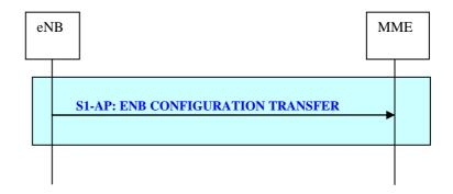
Figure 19.2.2.9a-1: eNB Configuration Transfer procedure
