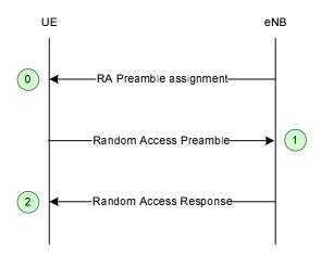
Figure 10.1.5.2-1: Non-contention based Random Access Procedure
