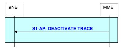
Figure 19.2.2.19.3-1: Deactivate Trace procedure
