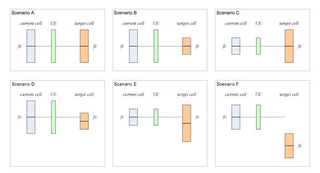
Figure 10.1.3-1: Inter and Intra-frequency measurements scenarios
