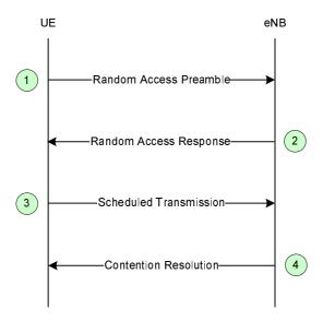
Figure 10.1.5.1-1: Contention based Random Access Procedure
