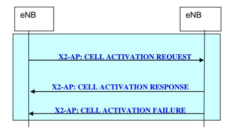
Figure 20.2.2.15-1: Cell Activation procedure
