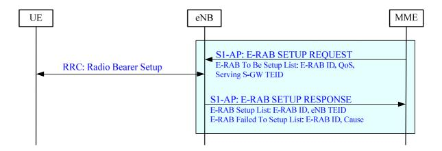
Figure 19.2.2.4.1-1: E-RAB Setup procedure
