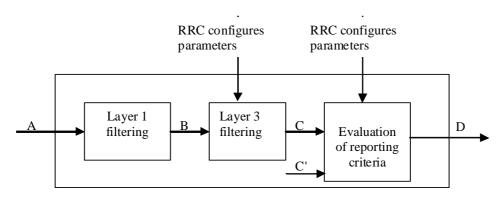
Figure 10.6-1: Measurement model
