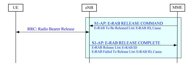
Figure 19.2.2.4.3-1: E-RAB Release procedure
