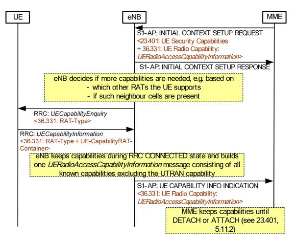
Figure 18-1: Initial UE Capability Handling
