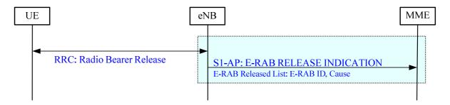
Figure 19.2.2.4.4-1: E-RAB Release Indication procedure
