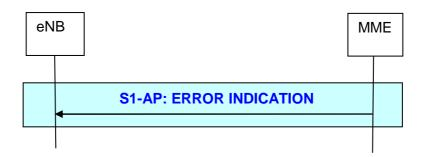
Figure 19.2.2.7.2b-1: MME initiated Error Indication procedure
