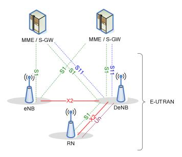
Figure 4.7.2-1: Overall E-UTRAN Architecture supporting RNs
