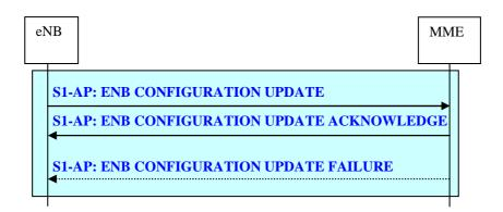
Figure 19.2.2.9-1: eNB Configuration Update procedure
